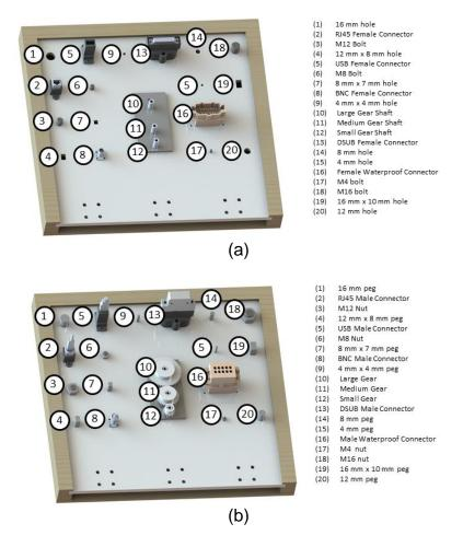
Figure 1: (a) Task board and base parts prior to assembly, (b) Fully assembled task board
