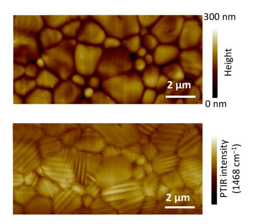
**Top:** Image recorded by an atomic force microscope reveals the topography of a polycrystalline sample of the perovskite, including the boundaries between crystals. **Bottom:** Image taken with the photothermal induced resonance technique shows the newly discovered ferroelastic domains (striations) within most crystals. Scale shows the PTIR signal intensity, a measure of the infrared light absorbed by the sample. Credit: NIST
