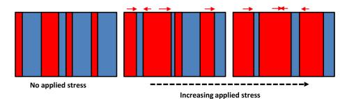
Illustration shows that in response to an applied stress, such as bending, the boundaries of the ferroelastic domains (red and blue regions depict domains oriented in different directions) become
