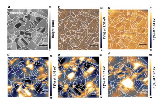
Topographic image (a) of the thin slice of a cadmium-telluride sample and images (b-f) of same slice taken with the direct-transmission near-field scanning optical microscopy technique. Credit: Yoon et al./NIST
