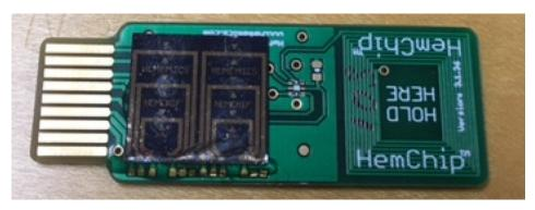
Image of full chip that can detect bacteria in less than 30 seconds. Credit: HeMemics Biotechnologies
