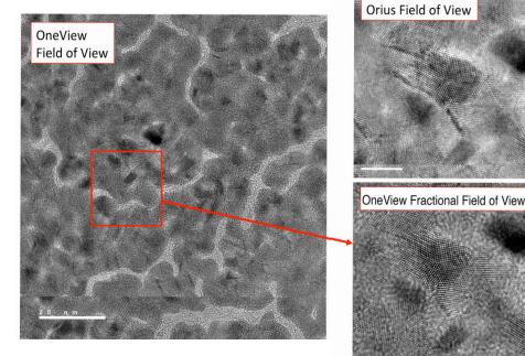
**Left:** Full field of view on the new TEM camera shows gold on a carbon support film. Due to the large field of view and small pixel size of the camera, columns of gold atoms can be observed everywhere in the image when viewed at full resolution (bottom right image). **Right:** The field of view of the old camera (top), which still operates on the TEM, covers only a fraction of the new camera's field of view (bottom). Credit: Alline Myers/CNST
