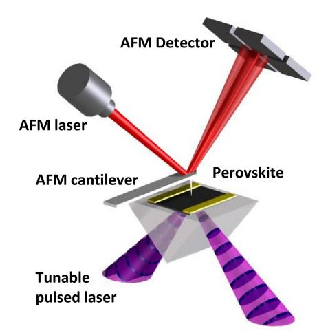
Schematic shows a perovskite sample (black) examined by the photothermal induced resonance technique. When the sample absorbs pulses of light (depicted as disks in purple cones), the sample expands rapidly, causing the cantilever of an atomic force microscope (AFM) to vibrate like a struck tuning fork. The cantilever's motion, which is detected by reflecting the AFM laser light (red) off the AFM detector, provides a sensitive measure of the amount of light absorbed. Credit: NIST
