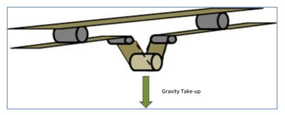
Figure2. Counter-weighted or Gravity Take-up Device
