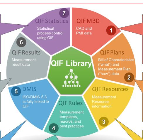
QIF MBD is the base for providing traceability to authority CAD data. It is not required for basic QIF use cases. Considered to be the strongest semantic CAD+PMI standard available
