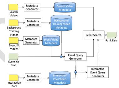
Figure 1: MED System Block Diagram: The MED processing modules are shown in blocks and data is depicted as icons. Folder icons represent a collection of videos while text-folders are text/csv documents. Dashed lines in the diagram show the now deprecated Interactive query generation and search.
