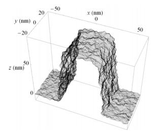
**FIGURE 1.** Line drawing of the roughest of our 3 virtual samples. The line is oriented to show the right edge. The left edge is obscured by absence of hidden line removal.
