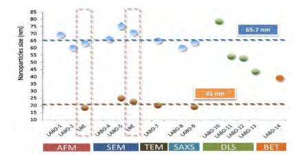
FIGURE 1. Measurements of nanoparticle size as a function of techniques used at different laboratories. Courtesy of Club Nanométrologie.
