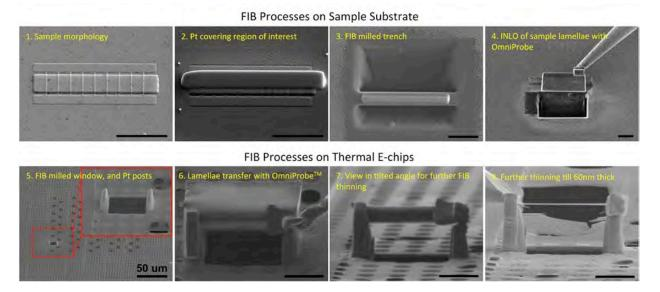
**FIGURE 1.** SEM images show the fabrication sequences to transfer the FIB cut lamellae from the home substrate onto the TEM membrane window of a TEM compatible thermal chip. All the scale bars are  $5\mu m$ , except the one labeled separately in step 5.
