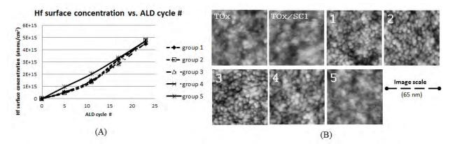
**FIGURE 2.** (A) Amounts of Hafnium deposited on ILs as a function of ALD cycles determined by RBS; (B) AFM images of IL surfaces with no  $HfO_2$  deposition together with those deposited with 5 cycles of ALD  $HfO_2$ , the labels on the top left corner provide the sample descriptions: TOx indicates the image is from the bare IL1 with no  $HfO_2$  deposition, TOx/SC1 indicates the bare SC1 treated IL1, the numbers indicate the images of 5 cycles of  $HfO_2$  from the 5 different sample groups.
