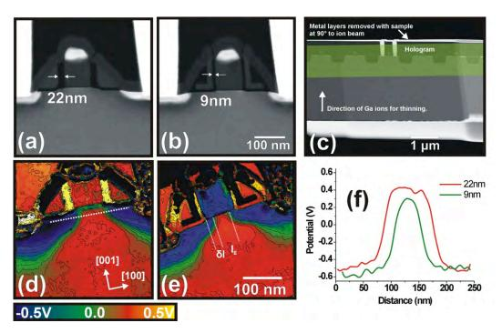
**FIGURE 1.** (a) and (b) show two p-MOS devices with different width spacers. (c) Electrically tested specimens have been prepared by back-side FIB milling. (d) and (e) show potential maps that have been acquired by off-axis electron holography. (f) Quantitative measurements of the electrostatic potential across the gate are shown.
