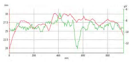
**FIGURE 5.** Line profiles of the AFM topography (red, left y-axis in nm) and the capacitance data (green, right y-axis in  $\mu V$ ) of the Device 6 area scanned in Figures 4 and 6.
