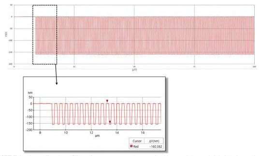
FIGURE 1. The small-scale profiling using XY scanner. The range is 100 um and the step height is 160 nm. The inset shows a magnified section of the same profile.
