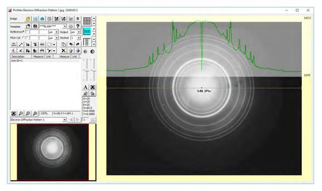
FIGURE 6. Electron diffraction image of microcrystalline specimen. [6]
