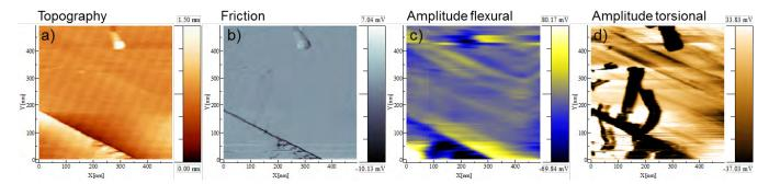
**FIGURE 2.** 492 × 492 nm<sup>2</sup> scanning probe images of the same area of a graphite sample displaying different signals. a) Topographic image taken at 280 nN applied normal (set-point) force; b) Friction (lateral force) signal image; c) Amplitude of the flexural response of the cantilever, demodulated at 1.65 MHz and d) amplitude of the torsional response of the cantilever, demodulated at 3.94 MHz. Dislocation system can only be distinguished at image d), by the dark lines.
