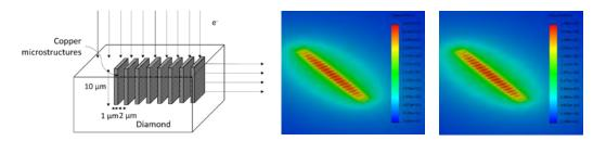
**FIGURE 5**. Scheme of the microstructured target of the Sigray Fine Array Anode Source Technology (FAAST<sup>TM</sup>) source (left) as well as thermal modeling of the Sigray FAAST<sup>TM</sup> (middle) and of a conventional Cu X-ray target (right)
