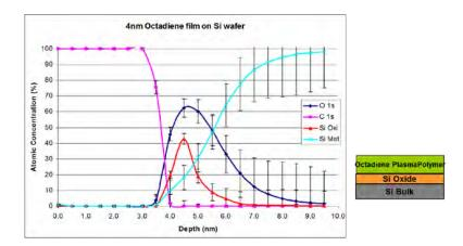
FIGURE 1. Maximum entropy modeling results from ARXPS data from an oxtadiene plasma polymer film deposited on the native oxide of a silicon wafer.
