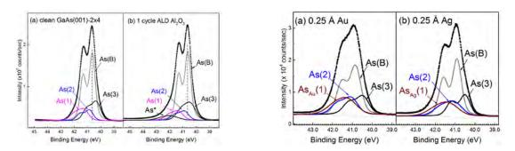
**FIGURE 1.** (Left) A fit to As 3d core-level spectra. (a) clean GaAs(001)- $2\times4$  and (b) 1 cycle of ALD Al<sub>2</sub>O<sub>3</sub> on GaAs(001)- $2\times4$ . **FIGURE 2.** (Right) A fit to As 3d core-level spectra. (a) 0.25 Å of Au and (b) 0.25 Å of Ag on GaAs(001)- $2\times4$ .
