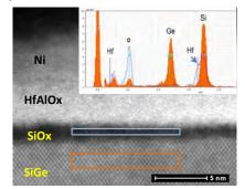
**Figure 4: STEM-EDX characterization of Al<sub>2</sub>O<sub>3</sub>-HfO<sub>2</sub> alloy/ Si<sub>0.7</sub>Ge<sub>03</sub>(001)/Si(001). Blue box shows a region of interlayer for EDS revealing a Ge-free SiOx interlayer. The orange box is a control region in the SiGe. The EDS spectra of the interlayer is in blue while the spectra on the SiGe control region is in orange. Note the absence of Ge in the interlayer.**
