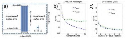
**FIGURE 2.** a) Initial proposed in-die target design (to scale) based upon the measured target from Ref. 1. The target has 30 lines with 60 nm pitch and line length  $(l_y)$  of 6  $\mu$ m. A three-dimensional electromagnetic scattering model was used to determine the minimum line length for maintaining accuracy. b) Dependence of the estimated uncertainties on the number of lines. c) Dependence of the estimated uncertainties on the number of focus positions. Panel a) reprinted from Ref. 3.
