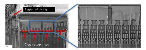
FIGURE 1. SEM cross-section images with crack stop structures of an Intel processor with 12 Cu metallization layers
