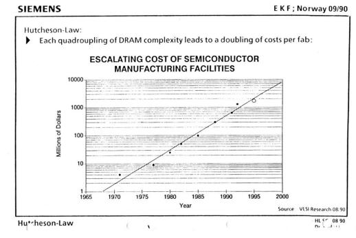
FIGURE 3. Fab cost escalation becomes a major fear in the early nineties, driving an intense need for process diagnostics.<sup>4</sup>
