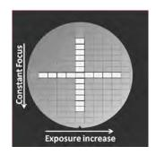
FIGURE 1. Wafer map for lamella prep used for both Wafer1 and Wafer2
