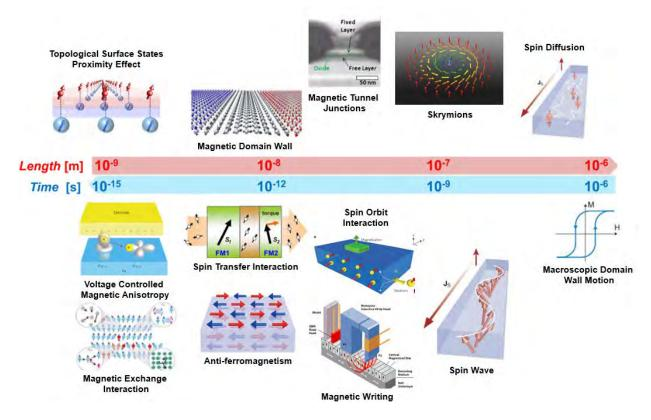
FIGURE 1. Various fundamental spin interaction mechanisms and spintronic devices in time and length scales. Revised from [3].
