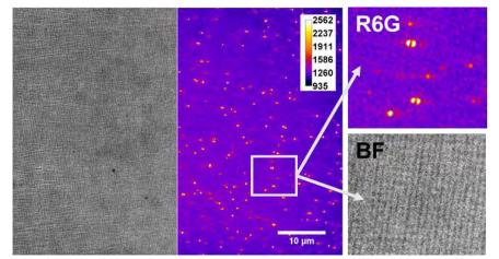
**FIGURE 1.** Bright field and false-colored fluorescence image (100xOI objective, 10 sec. exposure) of a plasmonic grating with a spin-casted 33 nm thin fluorescent PMSSQ film (10-14 M R6G) with expansions of the same location.
