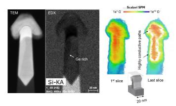
**FIGURE 10.** TEM, EDX and SSRM comparison for the same fin: the chemical analysis clearly reveals the presence of an extended defect in the (RSB) SiGe layer, where a Ge-rich area appears by the chemical EDX composition. A direct comparison with 3D SSRM of the same structure reveals an enhanced conductivity extending in the area across the 3D tomogram. Thus representing a potential threat for the off-state leakage of the transistor for the formation of parasitic paths under the finFET channel.
