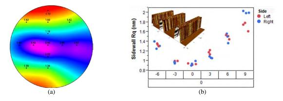
FIGURE 6. (a) Wafer map of sidewall RMS roughness and (b) their value change on Y axis of wafer
