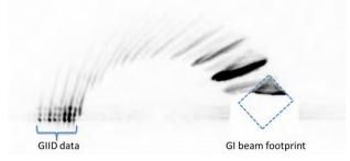
**FIGURE 2.** CCD detector image of data collected on a NIST Si Fin structure using the CLS to explore a new method for GI in-plane diffraction (GIID). The CLS beam was focused at the sample with a K-B multilayer (shown as a footprint of direct GI beam outlined in the box). The sample is rotated in-plane to reveal strong scattering resonances near grazing incidence. Note the sample itself is acting as an angular filter.
