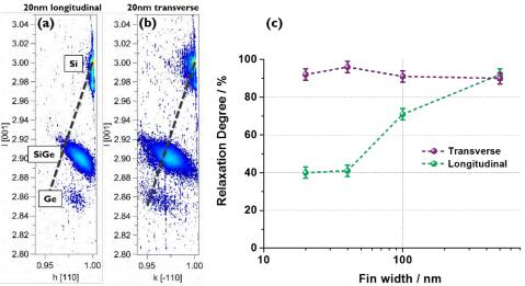
**FIGURE 1.** Reciprocal space maps (RSM) in the vicinity of the asymmetric (113) reflection acquired on 20nm wide fins in (a) longitudinal and (b) transverse direction. The dashed line in the RSMs connects the Si substrate peak with the center of the Ewald sphere and corresponds to the line of full relaxation. (c) Relaxation of the SiGe buffer in the transverse and longitudinal direction for different fin widths.
