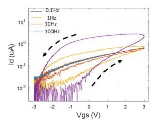
FIGURE 2. Experimental Id-Vg characteristics of polar polymer-based FeFET. 15 nm CP1 layer is incorporated as gate dielectric with 15 nm thick poly-Si layer used as the channel. The direction of observed hysteresis loop is schematically shown by arrows.
