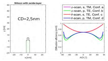
FIGURE 2. Numerical simulation of reflectance curves for a Si grating, period = structure height = 5 nm, CD = 2.5 nm
