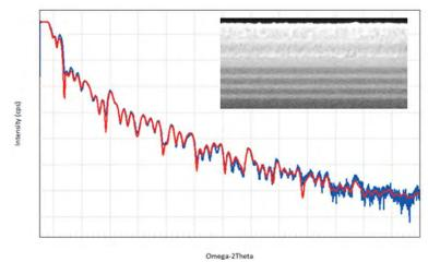
**FIGURE 2.** XRR from SiGe/Si nanosheet on a bulk Si substrate. Analysis of the measured data provides information on the individual layer thickness, density, and interfacial width (roughness). The measured intensity profile (blue) is overlapped with the best fit simulation (red). Comparison with a destructive SEM cross-section (inset) shows good thickness correlation.
