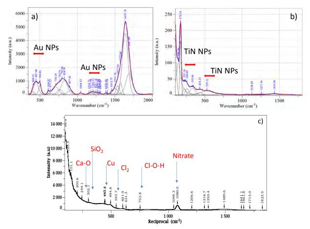
FIGURE 1. The spectra in a) and B) show the Raman modes of Au and TiN, respectively obtained from measurements in ultra-pure water. The known Raman modes for both materials are denoted with red arrows. The Raman spectrum in c) shows the Raman modes obtained from analyzing water as delivered from the municipality source and the contaminants that it contains.
