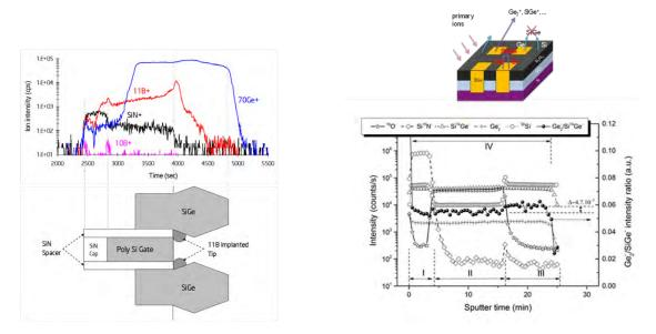
**FIGURE 2.** SIMS methods under development for measuring nanoscale device material parameters. 1.5D SIMS on left and Self-Focusing SIMS on the right [6].
