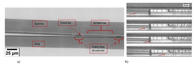
**FIGURE 3.** a) Stitched radiograph of a micro-DCB sample under load. The crack penetrates the crack stop structure from the chip side. The image is rotated clockwise by 90°, b) series of the virtual cross-sections based on nano-XCT, revealing the crack propagation at the Cu/low-k crack stop structure.
