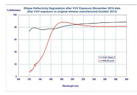
FIGURE 6. VUV degradation of the reflectance of protected aluminum. Unexposed sample (black); exposed sample (red).
