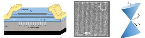
**FIGURE 2.** Left: schematic of electrostatic gating through a 1D superlattice. The top gate modulates the carrier density while the lower tunes the superlattice strength. Center: 20nm full-pitch superlattice of thin HSQ on top of SiO<sub>2</sub>. **Right**: highly squeezed Dirac cone demonstrating the anisotropic transport resulting from the 1D superlattice.
