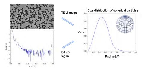
FIGURE 4. Data fusion of a direct (TEM) and an indirect (SAXS) measuring technique, giving rise to a new measurand, here the size distribution.
