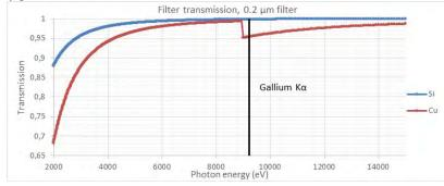
**FIGURE 3.** X-ray transmission trough a  $0.2 \,\mu m$  filter of silicon and copper. The black line indicates the Ka of gallium [8].
