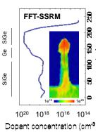
**FIGURE 8.** Due to the parasitic terms introduced by the small geometries (very high series resistance), FFT-SSRM is used for the direct quantification of the carriers in the SiGe-based raised S/D regions.
