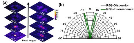
**FIGURE 2.** (a) Stacked fluorescence images taken at increasing focal plane height above the plasmonic grating. (Left) Angled SPCE and (Right) Airy disc pattern from the isotropic emission of a SM spreading with increasing focal height. Scale bar: 400 nm. Image exposure: 10 sec. (b) The normalized emission angle range for a SM of R6G plotted against the emission range predicted by the SPR dispersion and dye emission properties.
