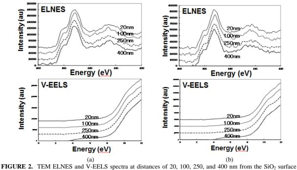
**FIGURE 2.** TEM ELNES and V-EELS spectra at distances of 20, 100, 250, and 400 nm from the SiO<sub>2</sub> surface without helium ions beam irradiation (a) and with  $2E14/cm^2$  helium ions beam irradiation (b).
