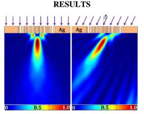
**FIGURE 2.** Focusing characteristics of the designed metalens. The intensity maps are obtained by setting the incident angles as (a)  $0^{\circ}$  and (b)  $30^{\circ}$ , respectively. Metalens height: 215 nm. Slit widths: 10-30 nm. Material in slits: air. All the sub-figures have been normalized by the maximal intensity.
