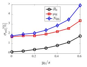
**FIGURE 2.** Relative standard deviation for  $R_0$ ,  $\mu_{\rm H}$  and  $N_{\rm HS}$  vs. width, w, of the test pad in question. The probe is placed at  $y_0 = 0.4s$  and the length, L, of the test pad is 7s. The relative standard deviation is seen to increase below w=3.5s.
