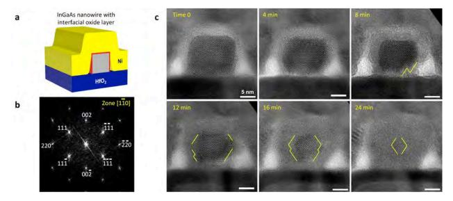
**FIGURE 2.** (a) schematic of Ni contacting with a InGaAs nanowire cross-section that sits on the  $HfO_2$  dielectric layer. (b) fast Fourier transform (FFT) image of the corresponding nanowire cross-section, showing the diffraction pattern along the zone axis
