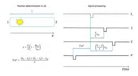
**FIGURE 1.** Position determination of ion hit in 1d case.  $t_i$  is the virtual signal denoting the real Time of Flight, channels 1 and 2 are two opposite outputs of meander wire.  $e^-$  is the electron start signal.  $t_m$  is the "meander time" associated with an imposed position dependent time delay on the actual ion arrival time.  $\Delta_{2,1}$  is the difference in time between signals on channel 2 and 1.
