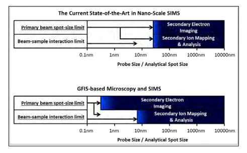
FIGURE 2. The applicable windows for Secondary Electron Imaging and Secondary Ion Mapping & Analysis.
