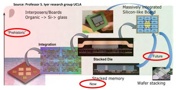
FIGURE 2. Evolution of System Level Heterogeneous Integration in a package
