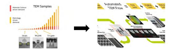
FIGURE 4. Technology driven increase in TEM sample output and the AutoTEM flow [5].
