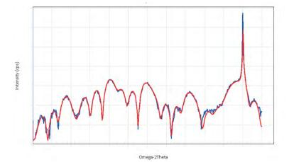
**FIGURE 1.** HRXRD  $\omega$ -2 $\theta$  scans around the symmetric (004) Bragg reflection from a SiGe/Si nanosheet on a bulk Si substrate. Analysis of the diffracted intensity distribution gives information on the lattice parameter of the individual layers with respect to the silicon substrate. Ge concentration and layer thickness are calculated from the best fit simulations (red) of the measured (blue) intensity profiles.
