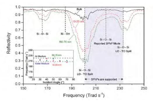
**FIGURE 1.** FTIR-ATR reflectivity of packed beds of 10-20 nm and 60-70 nm diameter  $SiO_2$  nanoparticles, and a bulk  $SiO_2$  film, vs frequency at an incident angle 70°
