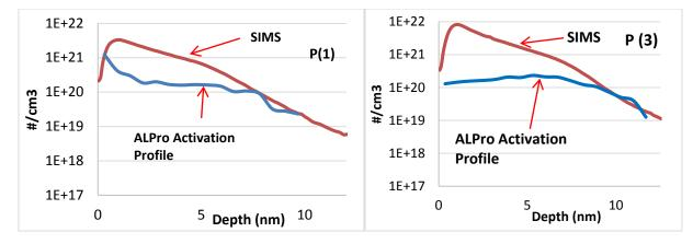
**FIGURE 1.** Samples:  $P1 = 1 \times 10^{15}$  cm<sup>2</sup> Phos-doped Silicon and  $P1 = 3 \times 10^{15}$  /cm<sup>2</sup> Phos-doped Silicon. The post-anneal SIMS 'as-is' dopant profile, and ALPro Activation profile.
