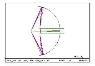
FIGURE 5. Two-mirror objective design.
