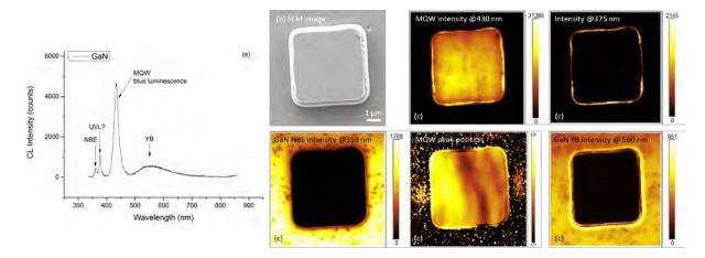
FIGURE 3. (a) Room temperature cathodoluminescence spectra showing all the emission lines. (b) SEM image of a single pixel. (c) Spectral maps of the different luminescence contributions.
