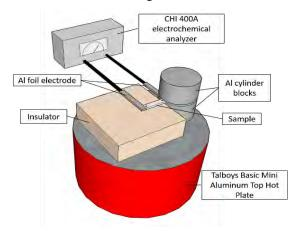
FIGURE 1. Schematic of the Self-built Seebeck Coefficient Measurement Apparatus.
