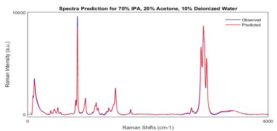
FIGURE 2. Raman spectra Measured for a mixture of IPA, DIW and Acetone. The measured and predicted spectra are compared.
