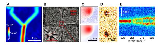
FIGURE 2. Examples of imaging nanomagnetism by NSDM: (A) Image of current density in a 50x50 nm<sup>2</sup> Pt nanowire [5], (B) Image of magnetic vortex in a 50 nm thin film of Fe<sub>20</sub>Ni<sub>80</sub> [6]. (C) Image of a single FeCo nanoparticle (experiment and simulation) [7]. (D) Image of magnetic noise from single superparamagnetic magnetite nanoparticles [9]. (E) Local field at a FeGe surface above and below the helimagnetic phase transition [9].
