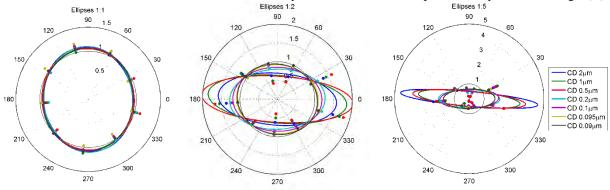
**FIGURE** 3 Polar plot of the normalized Rapid Nano signal for nine separate detection angles from Au ellipses of varying aspect ratios, for a number of different critical dimensions.
