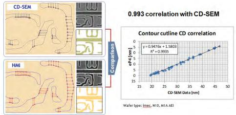
FIGURE 3. Benchmark with CD-SEM of cutline CD measurement on contour
