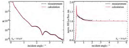
**FIGURE 1.** Comparison of conventionally modeled XRR of sample S4 800 °C (left side, Al<sub>2</sub>O<sub>3</sub> / HfO<sub>2</sub> / Al<sub>2</sub>O<sub>3</sub> layer sequence) and the resulting GIXRF signal (right side) for Hf in comparison to the experimental data.
