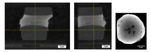
FIGURE 2. Three virtual 2D images (two perpendicular cross-section views and one planar view) through a solder connection (micro-bump of a HBM stack), based on a 3D data set from nano X-ray tomography. Imaging of a small extracted sample.
