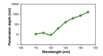
FIGURE 2. Penetration depth of silicon dioxide vs. wavelength. Note logarithmic vertical scale.
