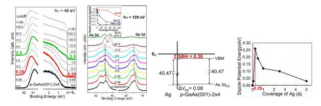
**FIGURE 3.** (Leftmost) Valence-band spectra in the vicinity of the Fermi level ( $E_F$ ) and low-energy cutoff recorded with a photon energy of 46 eV for Ag on a *p*-GaAs(001)-2×4 surface.
