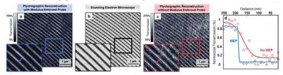
FIGURE 1. Ptychography CDI transmission image (a) reconstructed using the MEP technique, compared with an SEM image (b) and ptychography reconstruction obtained without the MEP technique (c). Lineouts (d) show 12.6nm resolution for the MEP reconstruction.
