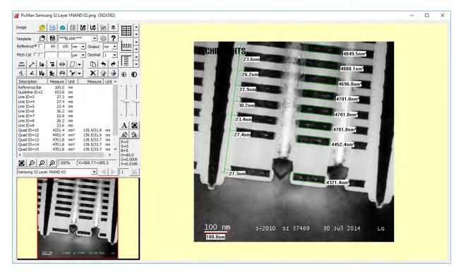
FIGURE 3. Cross section of a 3D V-NAND device (high magnification image). [3]
