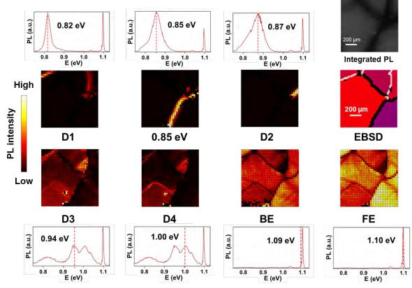
**FIGURE 4.**  $\mu$ PL intensity maps near sub-grain boundaries in "monolike" silicon showing the distribution of the well-known D-lines, the new line at 0.85 eV, the BE emission and the FE emission, on the same sample area at liquid helium temperature. Integrated PL map at room temperature and EBSD map are given on the same sample area. EBSD: white lines for low angle (<2 deg) disorientation, black lines for high angle (>2 deg) disorientation.
