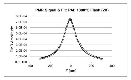
FIGURE 2. Exemplary PMR signal and fit for sample with PAI as a function of pump focal plane from sample surface.
