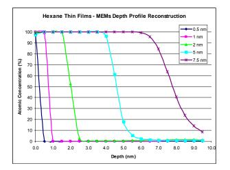
FIGURE 2. ARXPS/MEMs results from varying thicknesses of hexane plasma polymer films on silicon wafers, showing the thickness measurement capability inherent in the technique.
