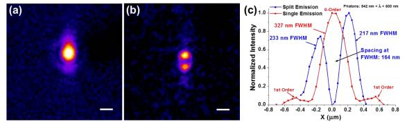
**FIGURE 3.** Background-subtracted Fluorescence images of single molecules of R6G on a plasmonic grating exhibiting a (a) diffraction-limited airy disc and (b) split emission due to SPCE. 100x Objective (NA 1.49), 10 sec. exposure, Scale bar: 400 nm. (c) Cross-section of the SM in (a) and (b) with calculated FWHM and separation distance of the split emission lobes.
