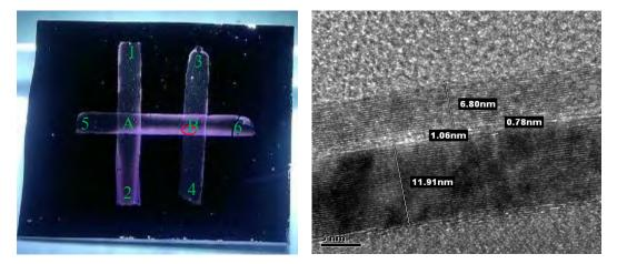
FIGURE 3. (a) Double-crossed graphene stripes (the numerical numbers are the probe locations) and (b) TEM cross-sectional image of contact B at the red circle indicated in (a).
