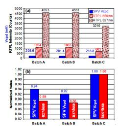
**FIGURE 1.** (a) average and (b) normalized Vcpd and RTPL intensity ratio (I827/I650) values over three 5-wafer batches (3 batches: 15 new blanket Si wafers).
