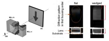
FIGURE 6. Crossed MLL after FIB preparation and assembly acting as a lens to image the object (OB) to the screen (SC) (left) [5] and diffraction patterns of flat and wedged multilayers (right).
