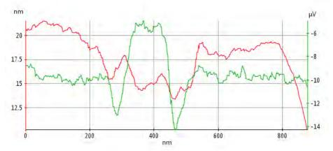
**FIGURE 2.** Line profiles of the AFM topography (red, left y-axis in nm) and the capacitance data (green, right y-axis in  $\mu$ V) of the Device 4 area scanned in Figures 1 and 3.
