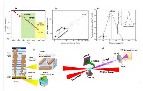
**FIGURE 1.** (a) Technology node versus year, indicating era of CD-SEM and future era of ICS CD-SAXS, (b) X-ray energy versus electron beam-energy [4, 6] (c) X-ray beam profile [4, 6] displaying the 65 keV band, (d) Various CD-SAXS and 3D tomography metrology applications in the integrated circuit, and (e) schematic layout of Inverse Compton scattering CD-SAXS beamline
