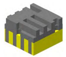
FIGURE 3. Simulation model of silicon dioxide (gray) over tungsten (yellow).
