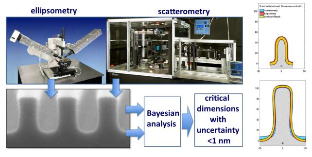
**FIGURE 1.** Left: scheme of a hybrid measurement approach: goniometric scatterometry and spectroscopic ellipsometry measurement data are combined in a Bayesian analysis to provide CD values with reduced measurement uncertainties; right: measurement results obtained with DUV (266 nm) reflectance measurements (blue), spectroscopic ellipsometry (red) and a hybrid analysis (yellow) of Si-gratings with nominal CD/pitch values of 25/50 nm (top) and 50/100 nm (bottom).
