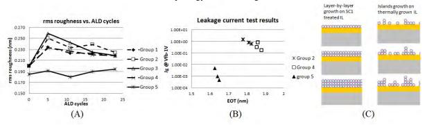
**FIGURE 3.** (A) rms roughness of the ALD  $HfO_2$  grown on the ILs; (B) MOS capacitor leakage current (Jg) and EOT test data from 23 cycles of  $HfO_2$  deposition on different types of ILs; (C) Growth model of ALD  $HfO_2$  on different ILs
