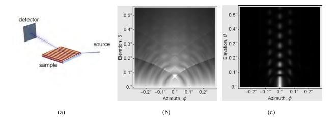
**FIGURE 2.** (a) schematic of simulated RSAES geometry. (b) simulated spherical wave RSAES pattern from line grating. (c) simulated vertical slit-aperture RSAES pattern from line grating.
