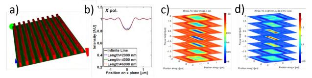
**FIGURE 3.** a) Single realization of a rough 10-line structure. b) Comparison between the profiles of the infinite and finite lines for three different line lengths  $l_y$  for a 10-line target at  $\lambda = 450$  nm. c) Images of the ideal, i.e. non-perturbed 10-line structure at several focus positions. d) Relative difference between the image of ideal and rough 10 line structures at several focus positions.
