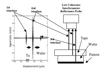
FIGURE 1. Measured asymmetric interferogram exhibits strong peaks corresponding to boundaries in the measured structure.
