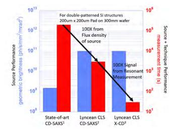
**FIGURE 3.** Comparison of raw source performance (left axis) and CD measurement time (right axis) for a 200um x 200um measurement pad on a 300mm wafer.
