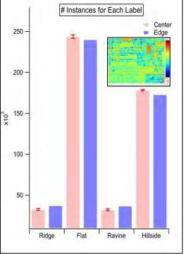
**FIGURE 3.** Surface patch labels for a test structure (inset) whose characteristics are known. Note the peak (1) at the center and ridges (2) and ravines (5) in concentric regions.
