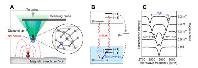
FIGURE 1. Basic principle of diamond-based magnetic sensing. (A) Scanning probe with an NV center at its apex. (B) Electronic and magnetic level structure of the NV center. A microwave transition (blue) is exploited for sensing. (C) Typical fluorescence response of an NV center when subjected to microwaves. The frequency of resonance peaks directly give the value of the local magnetic field.
