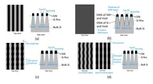
**FIGURE 1.** Different methods of including Line Edge Roughness are shown. 1.a shows idea lines with no LER. 1.b shows the use of and effective medium layer to model LER. 1.c shows a non-random sinusoidal line edge. This method proved to be the most successful 1.d shows a line segment off-set approach. [2]
