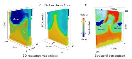
**FIGURE 3.** 3D-reconstructured volume of a single device visible at different stages along the y axis. (a) Out of the channel where the gate contact is visible and (b) under the gate where the spatial distribution of the S/D implants and the channel region are clearly visible. In addition, the other parts of the device are potentially accessible, for example in (c), filtering respectively the highest and lowest conductive features, the contact silicide and the spacer can be emphasized.
