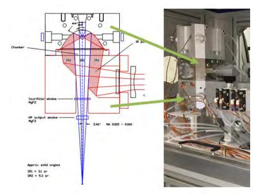
pump focusing and collection optics together and then seal this at the inputs and output. Figure 7 shows the configuration and example of a prototype lamp house designed with this implementation.
