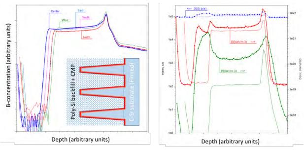
FIGURE 1. panel a (left): 1.5D SIMS B-profiles on Fin arrays from different wafer locations after Boron plasma doping and subsequent RTA, cleans / poly-Si backfill / CMP, and panel b (right): 1.5D SIMS N and O profiles on Fin array with (symbols) and without (no symbol) SiNx residual hardmask
