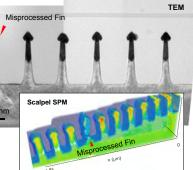
**FIGURE 6.** (a) STEM image of a single device with details of each element. In the table, the process flow used in the sGe pFinFET test vehicle. (b) Direct comparison of the same region as inspected by TEM (structural) and Scalpel SPM (resistance).
