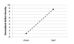
FIGURE 3. Defect densities after HCl etch
