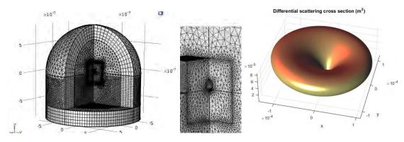
**FIGURE** 2 Geometry (left and center panel) and scattering profile (right panel) for typical RN3.9 illumination conditions. The differential scattering cross section calculated with an analytical model for a 30nm-radius spherical Au particle on a Si substrate illuminated by p-polarized light coming in at a 60° angle.
