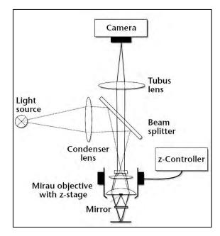
**FIGURE 1.** Optical path in white-light interference microscopy. (figure attributed to Polytec GmbH)
