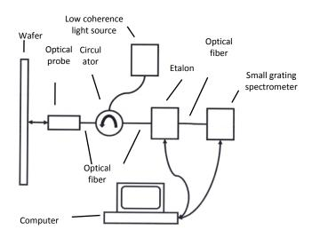
FIGURE 2. System enabling observation of Fabry Perot fringes in thick samples.
