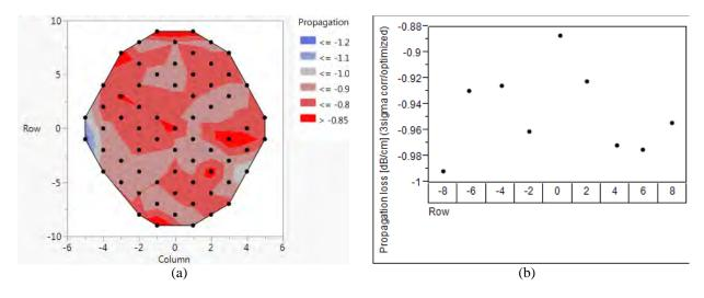
**FIGURE 7.** (a) Wafer map of propagation loss, measured at the wavelength of 1550 nm and (b) their value change on Y axis of wafer
