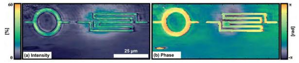
FIGURE 2. Reflection-mode ptychography CDI intensity (a) and phase (b) images of 29nm tall nickel structures on a silicon substrate.
