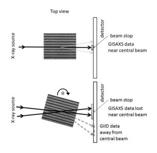
**FIGURE 2.** Top view of GISAXS vs. Grazing Incidence In-Plane Diffraction (GIID) configuration. On the left, GISAXS requires a collimated beam and fine alignment of features along the beam direction. A beam stop is used to prevent the detector from saturating in order to measure scattering. On right, rotating sample in-plane creates conditions for reflection from multiple GIID scattering sites in the sample. GIID can use a focused beam to significantly increase intensity on the sample.
