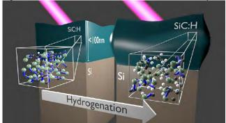
**FIGURE 1.** Artist's illustration of Coherent EUV Nanometrology. This study revealed increasing hydrogenation decreased average bond coordination and decreased compressibility in low-*k* SiC:H thin films<sup>2</sup>.
