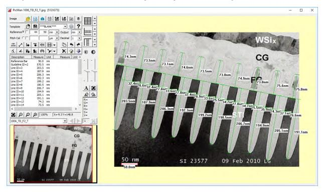
FIGURE 1. Dimension measurement example from a TEM image. [1]
