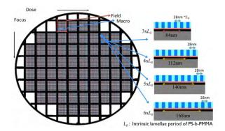
FIGURE 2. Line Space Block Copolymer arrays fabricated on a wafer with different focus-exposure conditions. The test areas contained sections (macros) with different guide structure pitches.[3]
