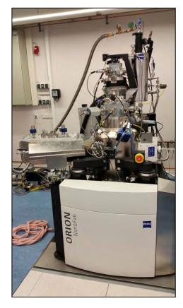
**FIGURE 1.** 3<sup>rd</sup> generation prototype of a GFIS based Microscope & SIMS combined instrument.
