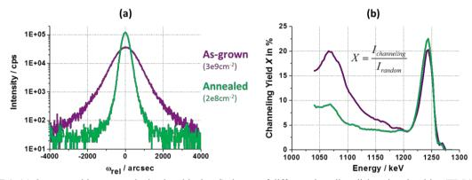
**FIGURE 1. (a)** Omega rocking curve obtained on blanket Ge layers of different threading dislocation densities (TDD). (b) RBS channeling yield measured on the same Ge layers.
