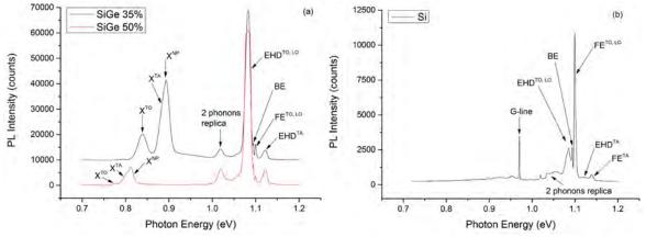
**FIGURE 2.** (a) PL spectra at 5K of Si/SiGe multilayers with 2 different germanium content. (b) Observation of the radiation-induced G-line after silicon etching (PL at 15K).
