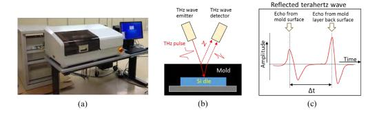
FIGURE 1. (a) TS9000 measurement unit (left side on the table), rack mounted controller electronics and optics (right), and controller PC (right side on the table). (b) Measurement configuration of overlaid mold thickness with pulsed THz radiation. (c) Example of reflected time-domain waveform from the DUT.
