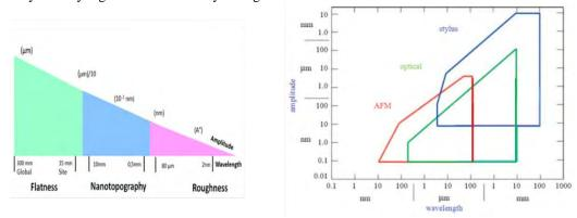
**FIGURE 1.** a) Nanotopography domain in spatial wavelength and amplitude; b) wavelength and amplitude of different surface topography instruments.
