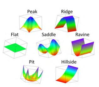
**FIGURE 2.** Surface patch labels. Pixels of 7x7 are classified according to characteristics.
