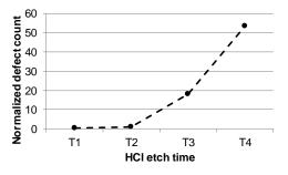
FIGURE 1. Defect count vs. HCl etch time
