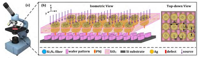
**FIGURE 1.** (a) Illustrated diagram showing a coherent optical microscope and (b) the mechanism of the metalens array-assisted defect detection system.
