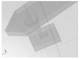
Figure 1: COMSOL generated image of the simulation geometry. A round base, conical tip (10  $\mu$ m in height), the conductive cantilever, and a two-line test structure are shown.
