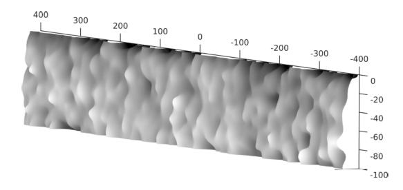
**FIGURE 3.** A three dimensional view of the boundary between exposed and unexposed resist. The surface is obtained from a simulated exposure of a 100 nm thick layer of CAR on an infinitely thick silicon substrate, assuming a Poisson distributed exposure dose of  $40 \,\mu\text{C/cm}^2$ .
