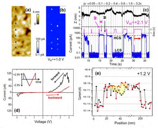
FIGURE 1. (a) constant-gap topograph (60x150 nm) and (b) corresponding current map at V<sub>R</sub> after series of 14 voltage pulses. (c) time evolution of current (blue) and the gap (black) in response to voltage pulses (magenta) with WRITE (W), READ (R) and move (M) phases for positions marked by 'x'. (d) I-V spectrum with a hysteresis loop. Insert shows applied voltage vs. time. (e) Variation of HCS-LCS current difference at +1.2 V as a function of position for two traces.
