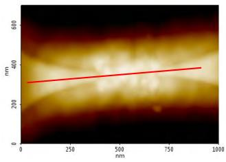
**FIGURE 4.** Contact mode AFM topography image of the second and malformed vacuum-channel device's (Device 6) sensordrain interface, vacuum-channel, and insulated gates region. The overlaid red line corresponds to the topography line profile displayed in Figure 5. Scan size: 700 x 1000 nm, image size: 290 x 200 px.
