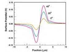
Figure 2: Simulated potential measurement across a test structure consisting of two lines, with the left line at negative potential and the right line at positive potential. The width of the response is related to the top cone width, while the slope of the response at the boundaries is inversely proportional to cone angle  $(5^{\circ}, 25^{\circ} \text{ or } 45^{\circ})$ .
