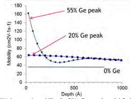
**FIGURE 2.** ALPro showed 70% increase in mobility for 20% Ge sample and 4.3x increase for 55% Ge sample 55% Ge sample concentration peak was at ~20 A (confirmed by AR-XPS)[6].
