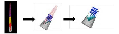
**FIGURE 3.** Atom Probe Tomography results highlighting localized 3D information from complex 3D nanostructures [5, 7].
