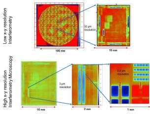
FIGURE 2. a) Low resolution Fizeau interferometer 100 mm scale data; b) Die level data extraction cm scale data c) high resolution PSI microscope Die level cm scale data d) in-die level μm scale data
