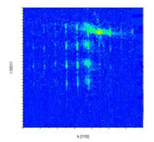
FIGURE 3. HRXRD reciprocal space map (RSM) in the vacinity of the 113ge Bragg reflection of fins etched into a nanosheet stack on Si(001) substrate.
