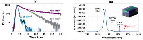
**FIGURE 2.** (a) Photoluminescence decay measured on thick relaxed Ge layers with different threading dislocation densities at 77K. (b) PL spectrum (77K) of an array of relaxed  $Si_{0.3}Ge_{0.7}$  fins (225nm wide) selectively grown in a STI matrix.
