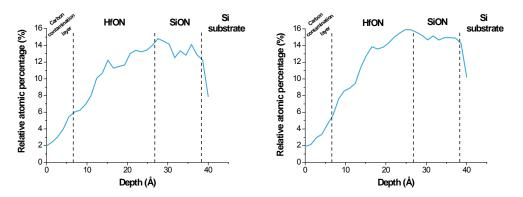
FIGURE 3. Nitrogen distribution obtained by chemical profile reconstruction from the pARXPS spectra (left) and the Nano-ARPES spectra (right).
