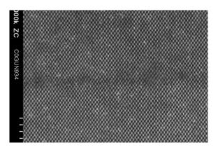
FIGURE 2: TEM micrograph of (bottom to top) Si, monolayer, overgrown Si; the crystallinity is clear, but where exactly is the interface?
