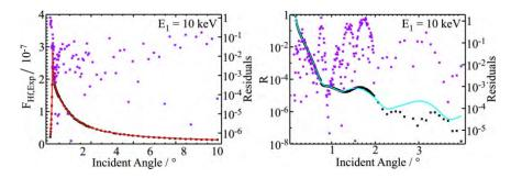
FIGURE 2. Results of the reference-free GIXRF-XRR (solid lines) for sample S5 ( $Al_2O_3 / HfO_2 / Al_2O_3$  layer sequence) in comparison to the experimental data (black dots). The residuals are also plotted as violet dots.
