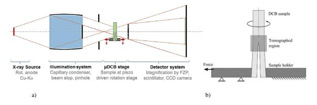
FIGURE 2. a) Scheme of microDCB test setup inside a nano-XCT tool, b) schematic drawing of microDCB test setup [1]
