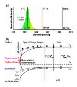
**FIGURE 2**. (a) spectral distribution of excitation light source and (b) schematic illustration of band bending with and without illumination.
