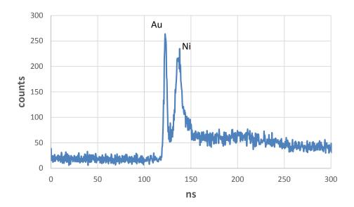
**FIGURE 2.** Time of flight spectrum of 0.7 nm Au on 2.7 nm Ni on Al<sub>2</sub>O<sub>3</sub> taken with a 10  $\mu$ m beam spot size and uncorrected for finite detector size and kinematic effects.
