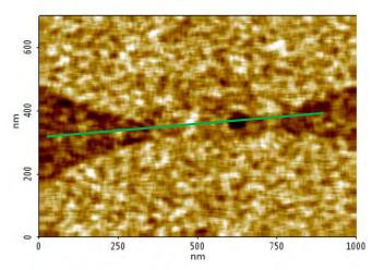
**FIGURE 6.** An SCM capacitance image of the region containing Device 6's sensor-drain interface, vacuum-channel, and insulated gates. Brighter colors correspond to relatively more positively charged areas on the device whereas darker colors correspond to relatively more negatively charged areas. Note the absence of electrical evidence for a functioning second
