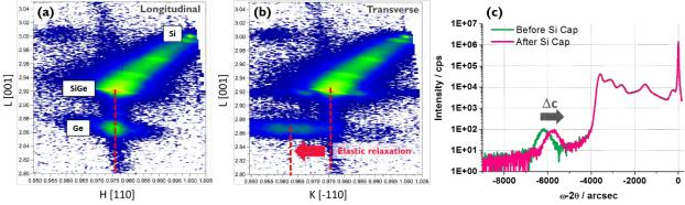
**FIGURE 2.** Reciprocal space maps (RSM) in the vicinity of the asymmetric (113) reflection acquired on 16nm wide fins in (a) longitudinal and (b) transverse direction. (c) (004)  $\omega$ -2 $\Theta$  scan reflecting the out-of-plane lattice parameter *c* measured before and after the conformal deposition of a Si cap around the Ge fin.
