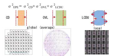
FIGURE 1. Edge placement error measurement requires global and local CD measurement
