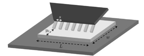
**FIGURE 1.** Illustration of an M7PP with 7 pins, separated by pitch *s*, placed on a rectangular test pad with dimensions  $L \times w$ , at a distance  $y_0$  from the insulating boundary.
