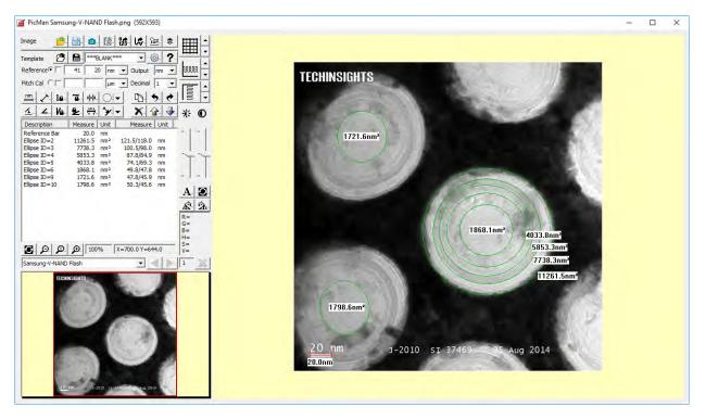
FIGURE 4. Plan view TEM image of 3D V-NAND device for area measurements. [4]
