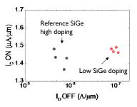
**FIGURE 12.** Impact of the SiGe SRB doping level (high vs low). In the low doping case, the formation of parasitic paths under the fin similar to the one presented here can induce a shift in the off-state leakage of the transistor.
