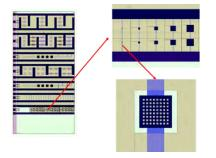
Figure 4: Section of test chip design with progressive enlargements showing the location of various sized 2-D electric tip profiler artefacts. Largest magnification shows buss structure, mid magnification shows different size 2D tip profilers, and highest magnification shows details of vias within a single profiler structure.
