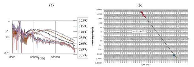
**FIGURE 1.** (a) Dependence of the measured imaginary part of the dielectric constant vs. frequency at different temperatures. MIM structure with 11nm thick CP1 was used. (b) Dependence of the peak frequency of the  $\varepsilon$ ''(*f*) spectra vs. 1/kT and the theoretical fitting to the experimental data (solid line). Expected value of peak frequency at room temperature is shown by the star symbol.
