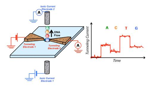
Illustration of experiment to directly identify the base pairs of a DNA strand (denoted by A, C, T, G in graph). Tunneling current flows through DNA placed between two closely spaced electrodes. Different bases allow different amounts of current to flow, revealing the components of the DNA molecule. Credit: J. Topolancik/Roche Sequencing Solutions
