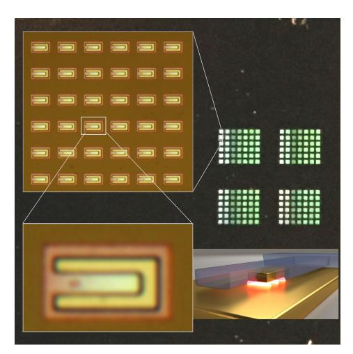
These optical micrographs provide a top-down view of several plasmonic gap resonators and zoom in on a single device. Bottom right shows schematic of a single device. Credit: Brian Roxworthy, CNST/NIST
