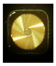
Semiconductor device, fabricated with the help of the NanoFab, designed to transmit high voltages. Credit: GeneSiC Semiconductor Inc.
