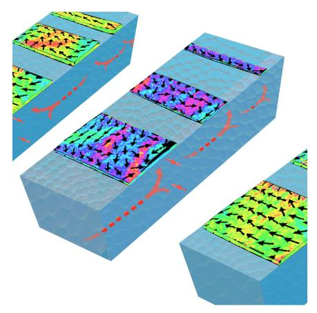
Strips of magnetic material (small colored rectangles) sit atop blocks of a nonmagnetic heavy metal (large blue rectangles). When an electric field is applied to a nonmagnetic block, a flow of spin-polarized electrons enters the magnetic strips and alters the direction of magnetization (black arrows). Credit: K.Dill/CNST
