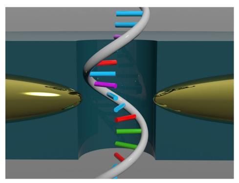
Schematic of DNA sandwiched between electrodes. Credit: From M. Di Ventra and M. Taniguchi, *Nature Nanotechnology* (**11**), 117 (2016)
