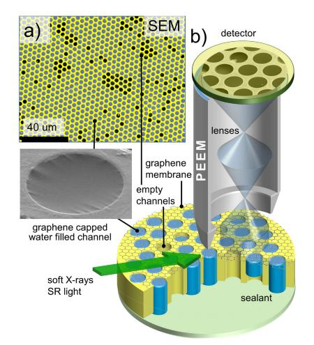
Experimental setup shows an array of graphene-capped liquids. The microcaps enable the liquids to be studied using an imaging technique that previously was restricted to studying solid surfaces. Credit: A. Kolmakov/CNST
