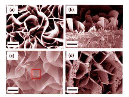
(a) SEM images of iron oxide nanoblades used in the experiment. (b) Cross-section SEM image of the nanoblades. (c) SEM image of nanoblades after 1 hour of reduction at 500 °C in molecular hydrogen, showing the sawtooth shape along the edges (red square). (d) SEM image showing the formation of holes after 2 hours of reduction. The scale bar is 1 micrometer. Credit: W. Zhu et al., *ACS Nano*
