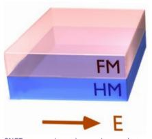
CNST researchers have shown that an electric field (E) applied to a layered structure consisting of a heavy metal (HM) and a ferromagnet (FM) creates a spin-polarized current generated at the interface between those materials. This spin current could be capable of flipping the magnetization of the ferromagnet. Credit: M. Stiles, V. Amin/ CNST
