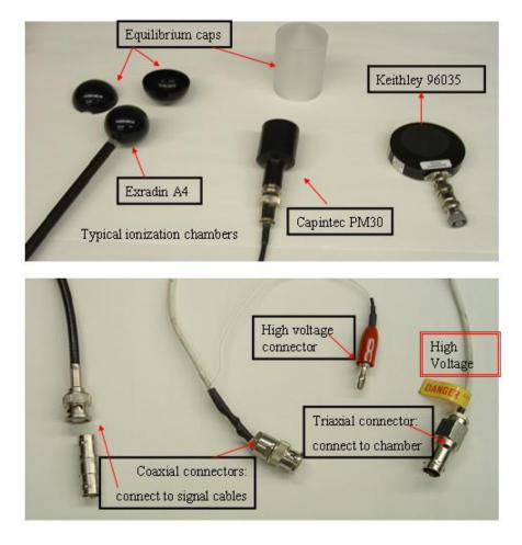
Figure 4. Typical chambers and connectors.
