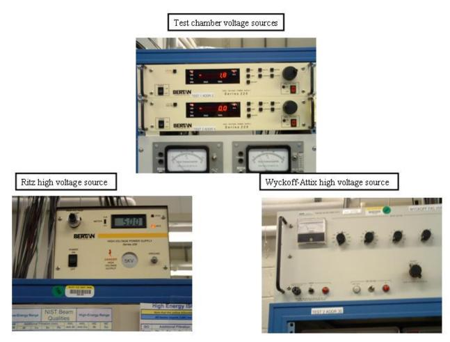
Figure 8. 100-300 kV high voltage power supplies.
