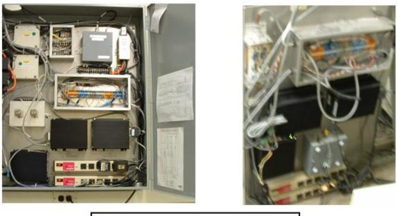
Motion control panels for the 100 and 300 kV range
