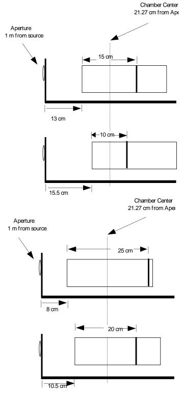
Figure 2. Typical Attix chamber configuration for air-kerma measurements.
