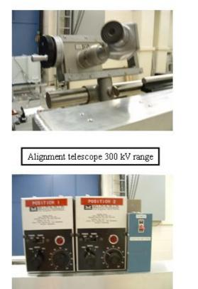
Chamber alignment controls 300 kV range
