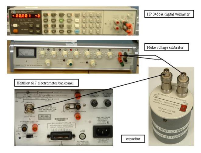
Figure 13. Electrometer calibration setup.
