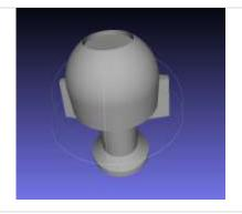
Figure 3 An design for the eye target blank which fits inside the face mount shown in Figure 2. The piezography printed pattern and cornea simulation solutions fits inside the front facing indentation in the design. The reflective properties of the 3D printed model is similar to that of the human sclara as seen in near-infrared wavelengths.
