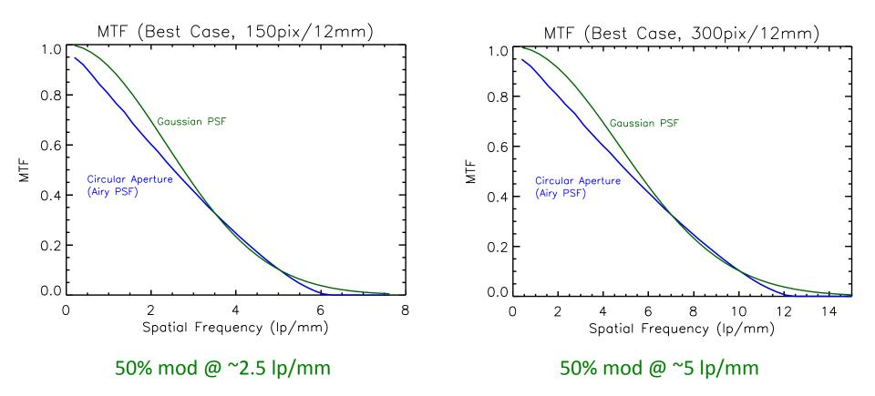
Examples from Best Case Diffraction Limited Conventional Optics (No Deconvolution)
