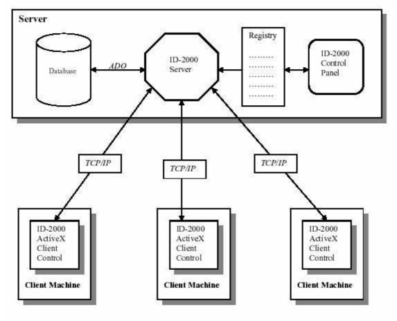
The ID-2000 SDK is modeled after the client-server architecture. An ID-2000 client connects to an ID-2000 server and asks the server to do something such as find a person or encode a face. The server fulfills the request and sends the results back to the client. Under the client-server architecture, the server, in response to client requests performs the majority of processing. The client-server architecture provides the following benefits:
