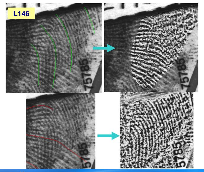
Current method requires manual input for undesired ridge lines (green lines on left top and red lines on left bottom).
