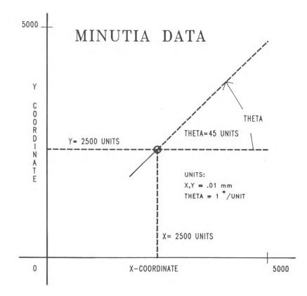
Figure 1 Minutia Coordinate System
