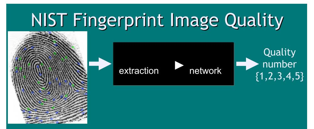
feature extraction: computes image content and fidelity characteristics and results in an eleven dimensional feature vector. neural network: classifies feature vectors into five classes of quality based on various quantiles of the normalized match score distribution.
