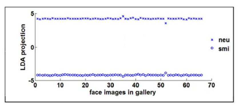
The LDA projection of all the gallery neutral faces used in this work has an average projection value of 4.2 with a small variance of 0.004; while the average LDA projection of the smiley faces is -4.2 with a small variance of 0.011.
