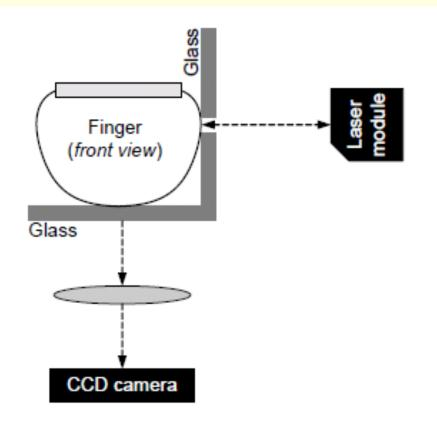
Laser measures the small changes in the skin due to the expansion and contraction of papillary lines
