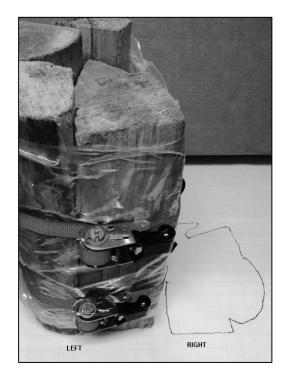
Figures 3-15. Tracing the Perimeter of the Wood.
