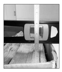
Figure 3-9a. Examples of the Headspace Measurement.
