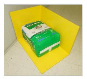
Figure 3-1. Dimensional Measuring Frame.
