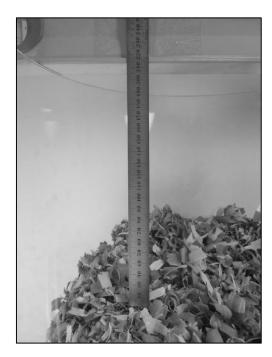
Figure 3-27. Ruler Shown with the Zero End at the Bedding Surface.
