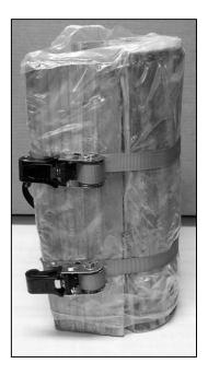
Figure 3-14. Bundle with Straps Placed at 10 cm (4 in).
