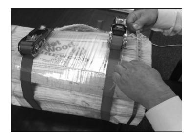
Figure 3-17. Strapping the Ends of a Bundle.
