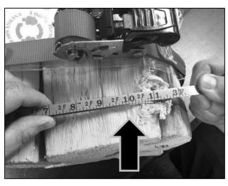
Figure 3-17a. Measuring the Circumference of the Bundle. At the point of the arrow, the circumference of the bundle is 2 ft 10 in (34 in).
