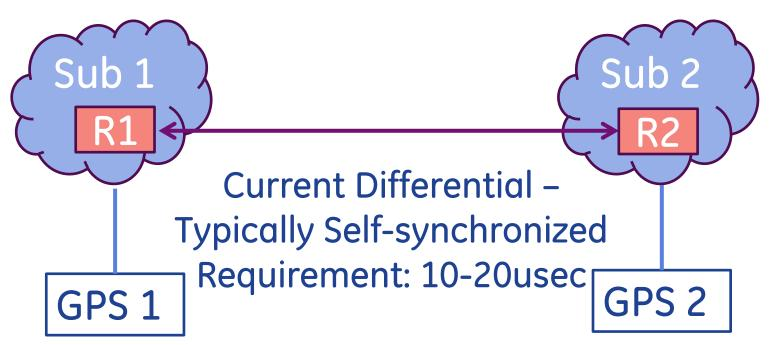
GPS Time Sync NOT needed nor desired.... ....unless Communication Paths are Asymmetric Problematic with Process Bus Data – given loss of Sync on one side
