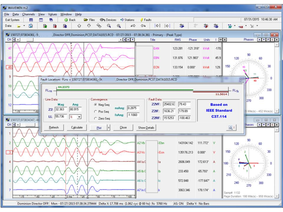
Lightning correlation (1 ms) - DFR data can be used to determine fault inception time which can then be used to determine if lightning caused the event by comparing our recorded event time to lightning strike data from a lightning service (FALLS - Vaisala).
