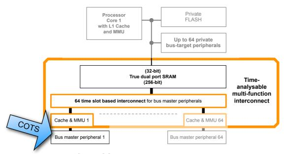
It is trivial to configure SSRT at design-time to ensure that each COTS bus-master peripheral has guaranteed wire-speed bandwidth with low latency
