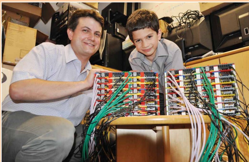
UK researchers have built an inexpensive supercomputer from a number of $35, credit-card-sized Raspberry Pi computers. The team was led by Professor Simon Cox, whose 6-year-old son, James, designed the Lego racks that held the Raspberry Pi units.
