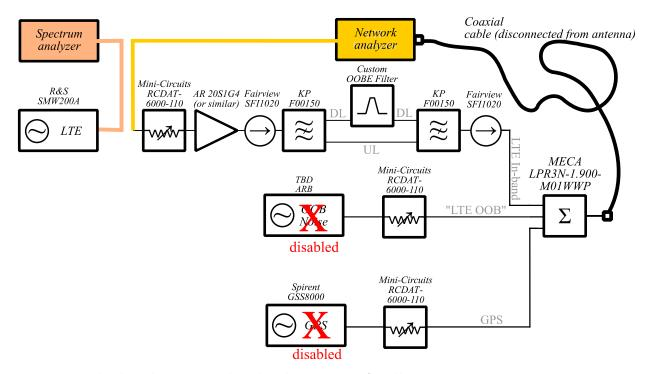
Figure 14. LTE in-band signal generation path conducted measurements for calibrations
