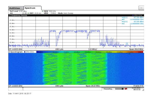
Figure 7. Example PSD measurement of a 10 MHz LTE uplink
