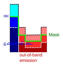
Figure 12. The in-band and out-of-band emission and the waveform mask for swept range emulation. The same losses apply to both in-band and out-of-band emissions.
