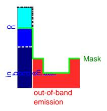
Figure 11. The in-band and out-of-band emission and the waveform mask for in-band LTE coexistence margin testing. Here, LTE out-of-band emission is held constant while LTE in-band emission is varied.
