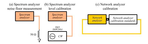
Figure 13. Instrument calibration signal paths
