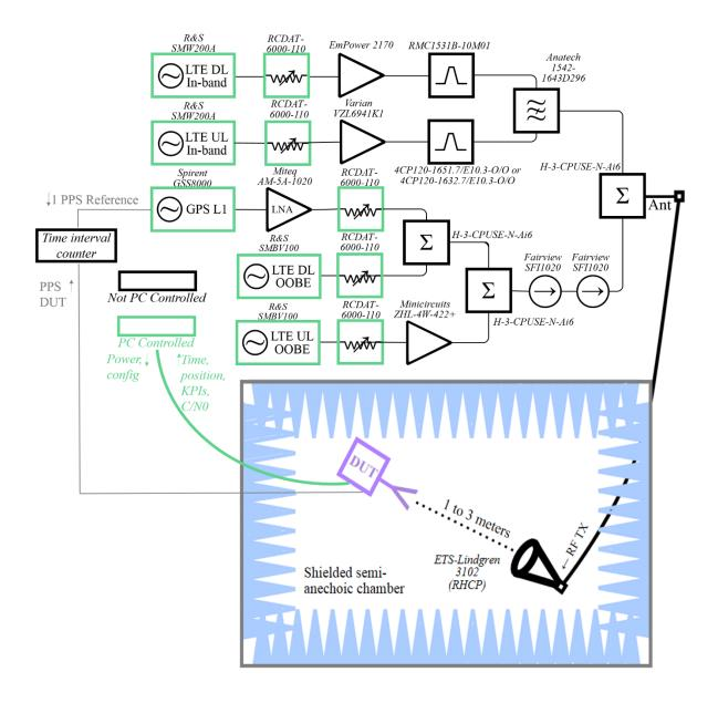
Figure 5 Setup for precision timing tests in the anechoic or semi-anechoic chamber.
