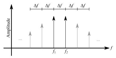
Figure 19. Center frequencies of intermodulation products
