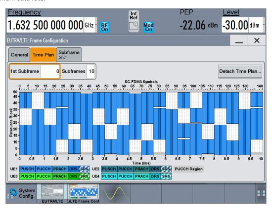
Figure 6. Example LTE uplink resource block allocation
