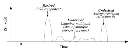
(b) Example field uniformity check by checking power levels in trainsformed "thru" measurements
