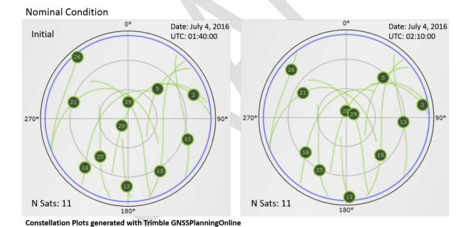
Figure 1. The Nominal satellite constellation. Initial GPS constellation (left), after 30mins (right). All satellites in view are configured to emit -128.5 dBm at the plane of the DUT assuming a 0 dBi receiving antenna.
