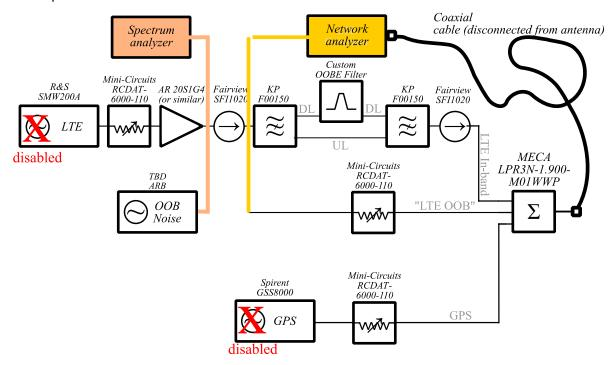
Figure 15. Conducted measurement setup for calibrating LTE out-of-band signal generation
