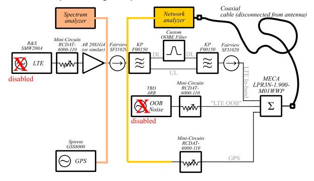
Figure 16. GPS L1 signal generation path conducted measurements for calibrations
