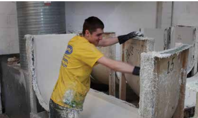
James Kilbane, an apprentice at MPM in Leeds, England, does hand layup on a bathtub panel.
