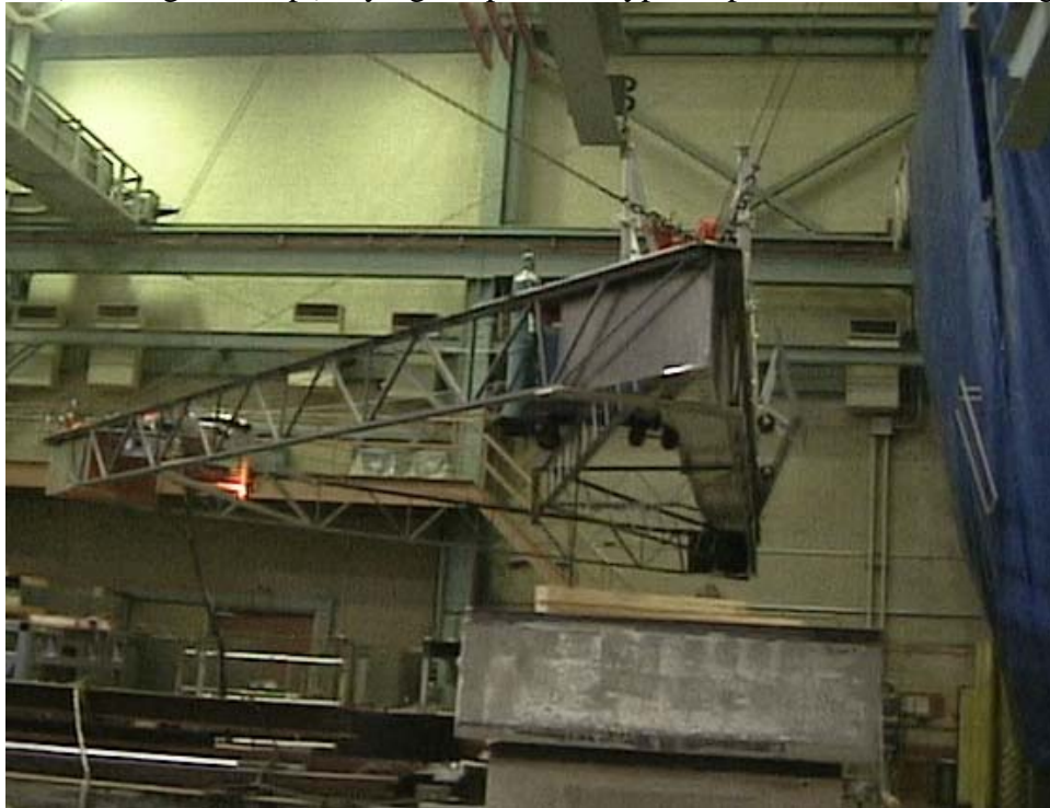
Full Scale (50' long x 22' dp.) Flying Carpet Prototype suspended in the NSIT high bay.
