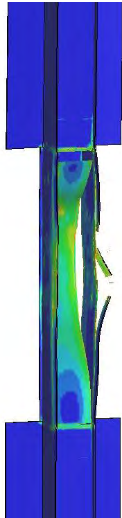
Fringes of Effective Plastic Strain.
