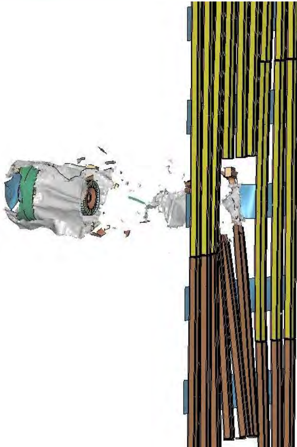
Spandrel Centered Impact
