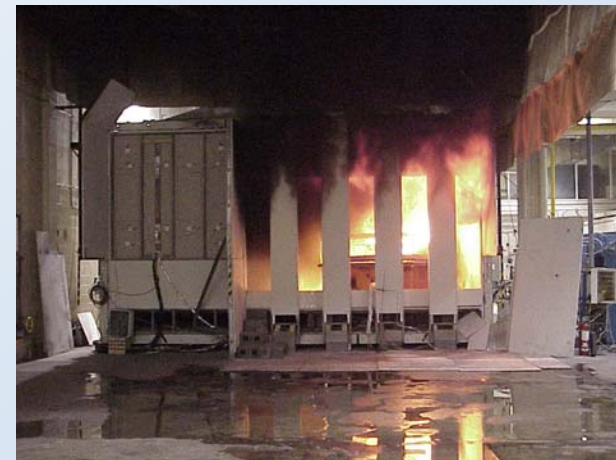
Multiple workstation burn tests for validation of fire model predictions
