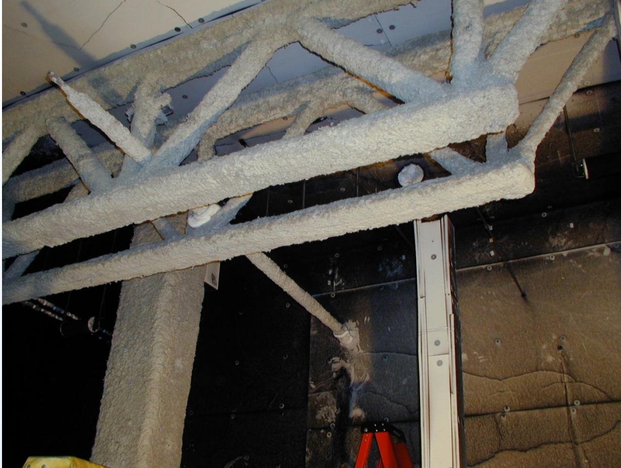
Figure 2. Insulated steel components in place prior to Test 5. In the foreground are two steel trusses and a steel rod, supported across the lower chord panel points, positioned near the ceiling above the fire pan. The steel column is located between the air inlet and the fire pan.
