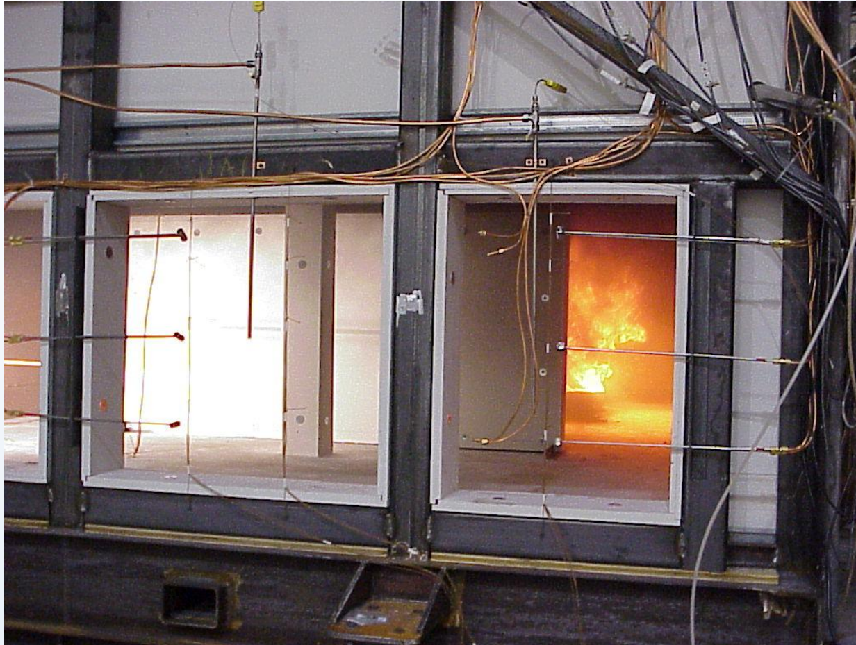
Figure 3. Inlet side of the compartment 5 minutes after ignition in Test 2. The fire is in the background. The foreground shows instrumentation for characterizing the air flow at the inlet. A baffle is located in front of the fire.
