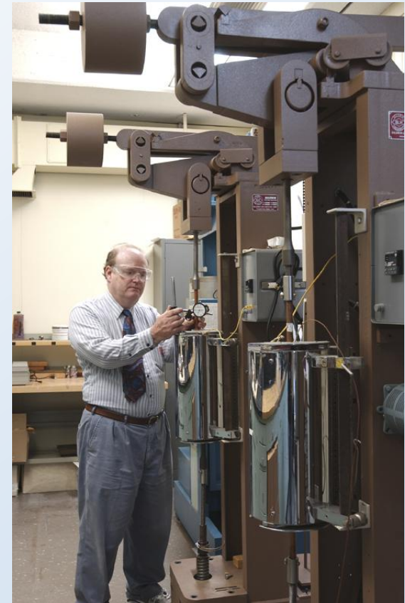
Adjusting a dial gauge on one of several creep testers that will be used to evaluate the high-temperature, time-dependent properties of WTC steel
