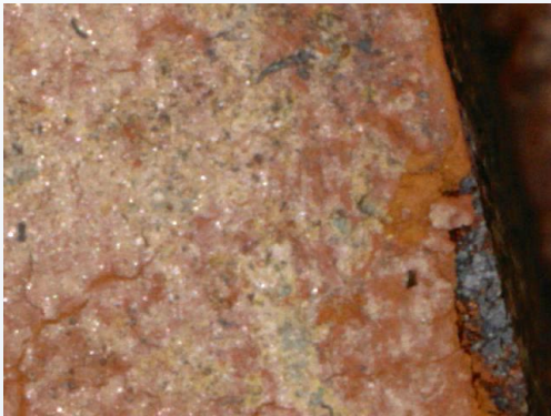
700 deg C for an hour mud cracks partially obscured by formation of whiteish "sandy" phase on surface delamination easy with finger
