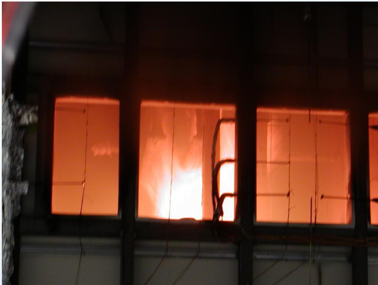
Figure 5. View of compartment from air exhaust outlet several minutes after the start of test 6. Note the flame impingement on the steel trusses and bar.
