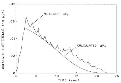
Fig. 2. Pressure difference,  $\Delta P_{li}$ , across the elevator lobby of a Toronto hotel due to piston effect. Conversion factor: 1 in H<sub>2</sub>O = 248.8 Pa.
