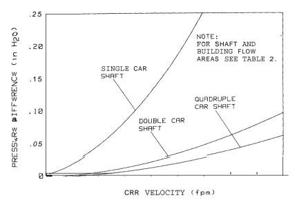
Fig. 3. Example pressure differences from building to elevator lobby due to piston effect. Conversion factors: 1 in  $H_2O = 248.8 \text{ Pa}$ ; 1 fpm = 0.00508 ms<sup>-1</sup>.
