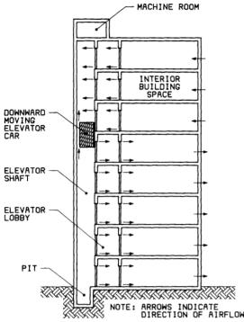
Fig. 1. Airflow due to downward movement of elevator car.
