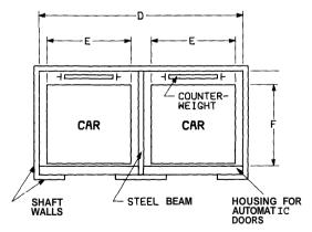
Fig. A1. Convention used for determination of A, and  $A_f \cdot A$ , = DG and  $A_f = DG - NEF$  where N = 1 for a single car moving and N = 2 for both cars moving together. Note that the area,  $A_f$ , does not include the small area between the car and the door housing because it is felt that the contribution of this area is insignificant.
