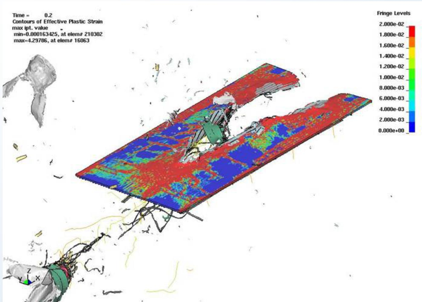
Fine Brick Element Floor Section Model
