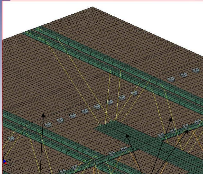
Smeared Concrete & Metal Decking Shell Model
