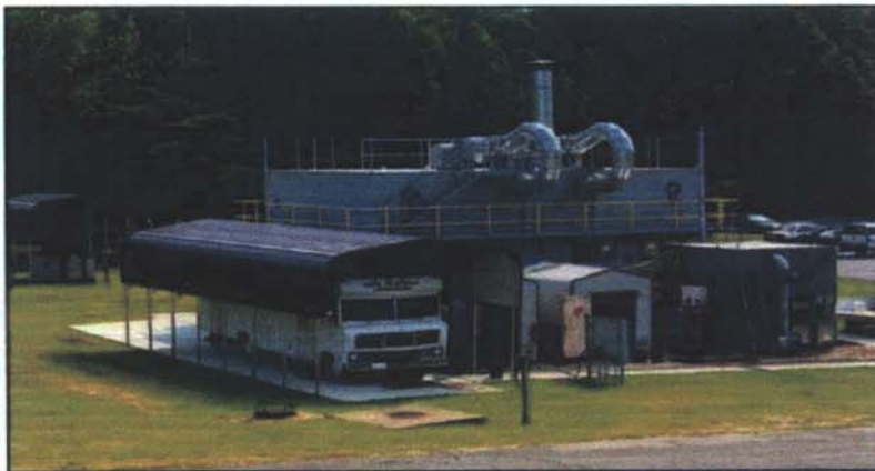
FIGURE 13 Fire test facility at the NRL Chesapeake Bay Detachment. The two enclosures at the rear (285 cubic meters) and the right (27 cubic meters) of the picture are used for testing different sized shipboard compartments.
