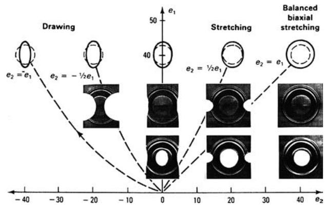
Fig. 1—Strain space description with images of the Raghavan-shaped specimen and matching washers.<sup>[6]</sup>
