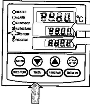
This operation is used to specify the automatic stop time in the fixed temperature operation mode.
