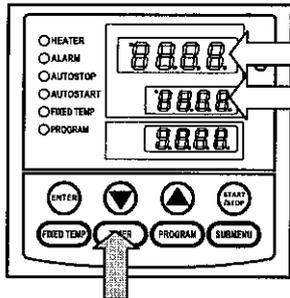
This operation is used to specify the period to automatically stop during operation.
