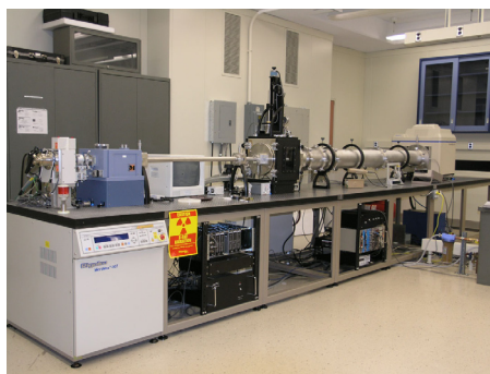
NIST designed x-ray scattering tool configured for small angle scattering with the Cu x-ray tube
