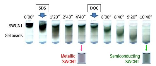
Figure 1. Pictures of continuous agarose gel beads separation of SWCNTs.
