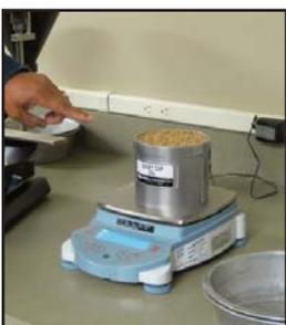
**Figure 4. Weighing the quart kettle and grain.**
