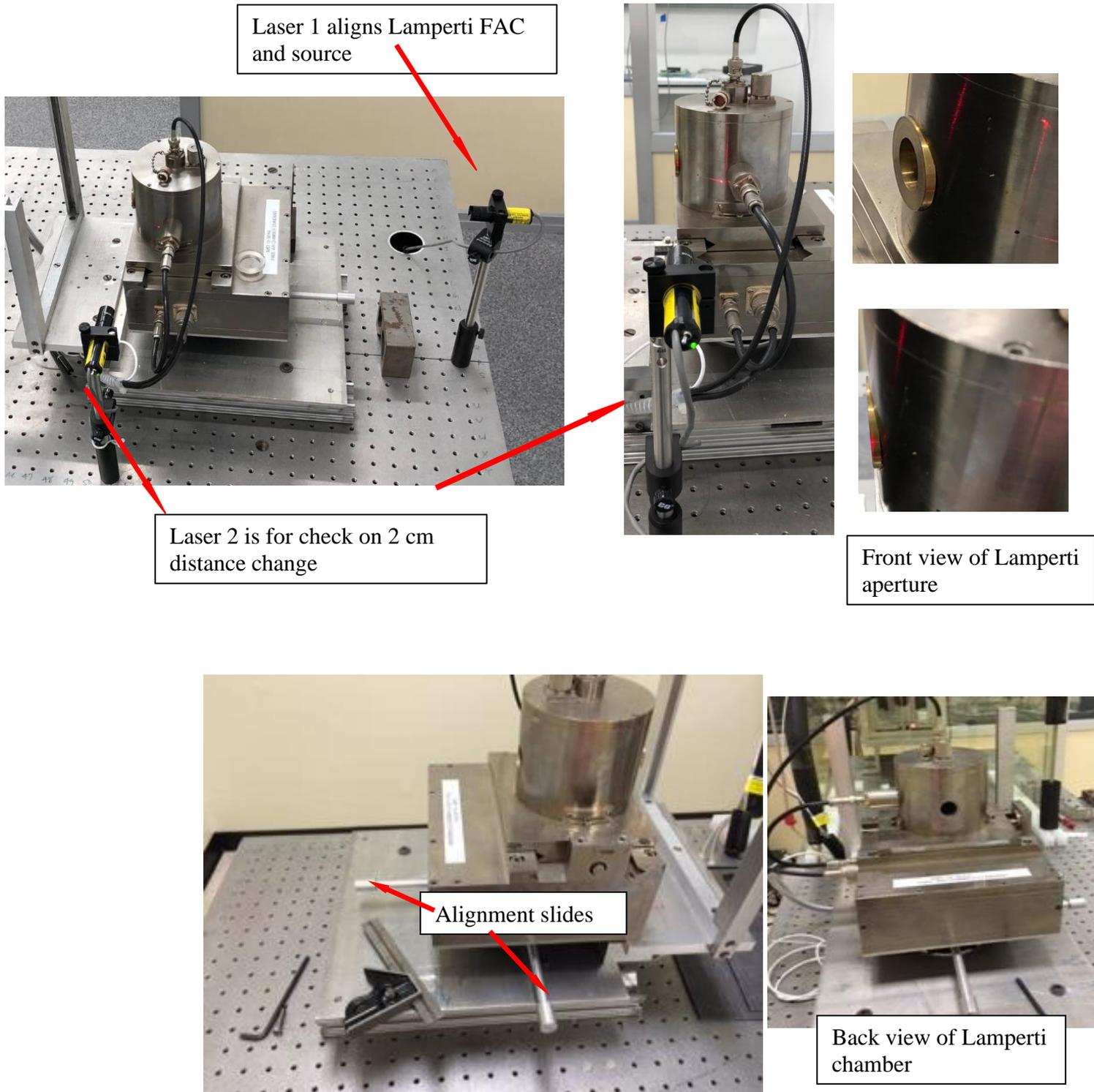
Figure 12. Techniques for Lamperti chamber and source alignment
