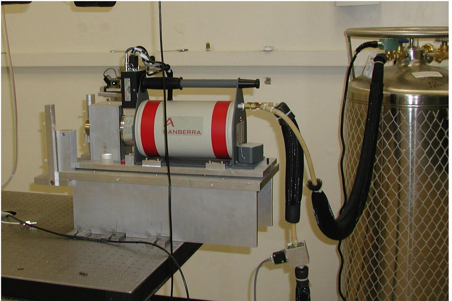
Figure 5. High-purity germanium detector with cooling Dewar.
