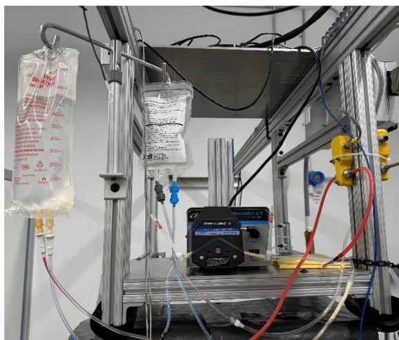
Water IV bag shown on left and Golden coolant on right. The red hose is to water flow switch. The flow switch cable attaches to the switch
