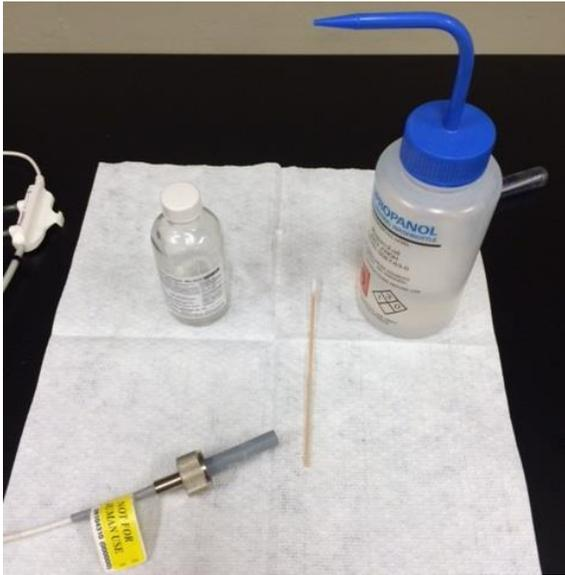
Figure 9. Supplies for cleaning HV connector, lubricant and isopropyl alcohol
