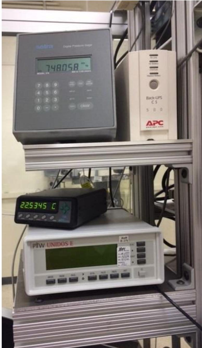
Figure 7. Barometer, thermometer and well-chamber electrometer.
