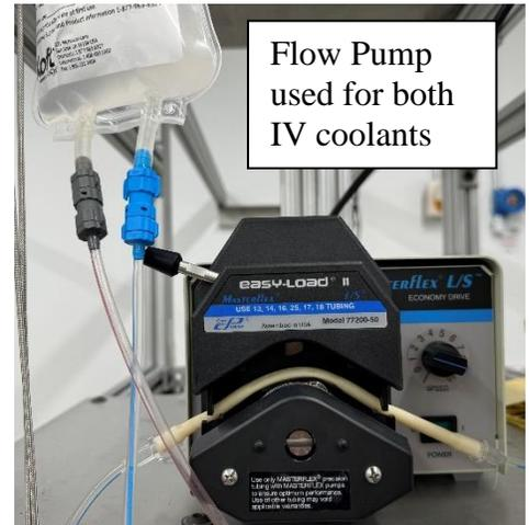
Flow Pump used for both IV coolants
