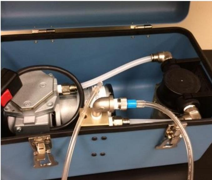
Figure 10. Vacuum pump and drying details.
