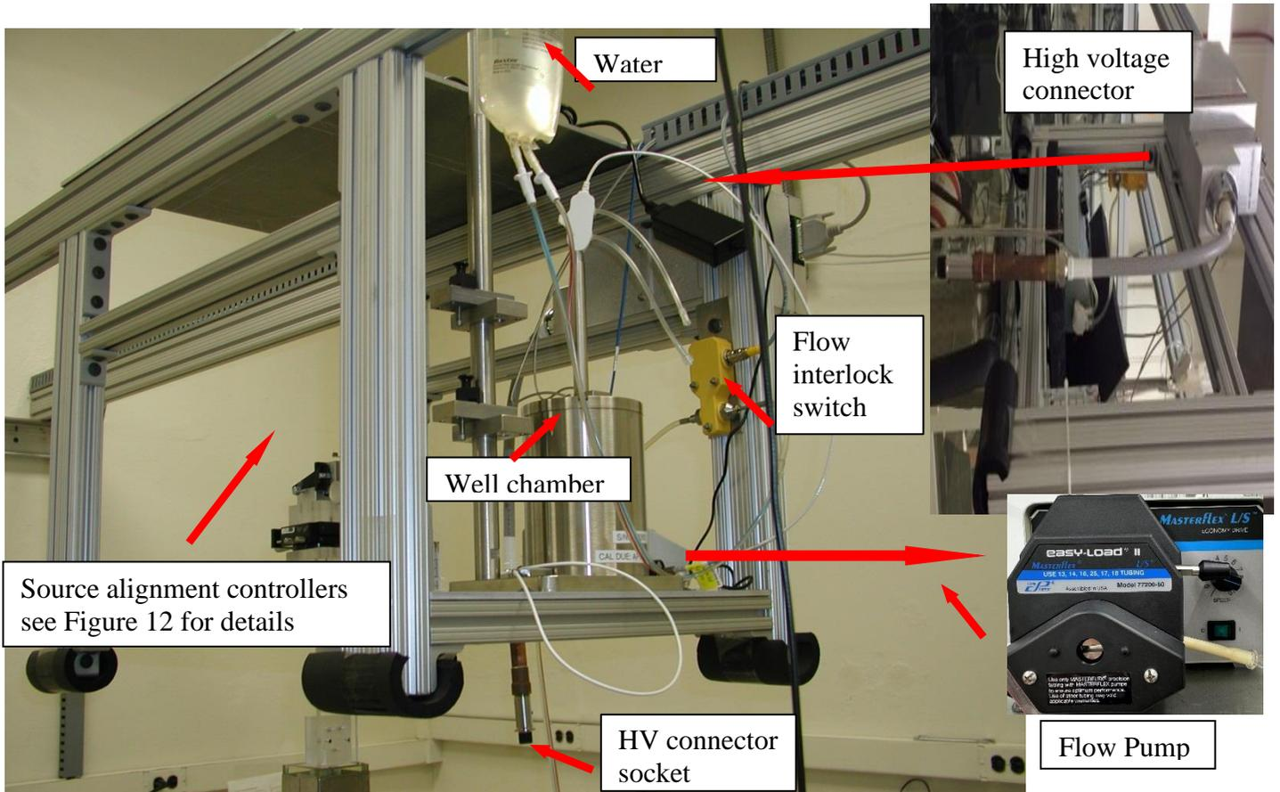
Figure 4. Well-chamber platform with water IV bag, flow pump, shown in smaller picture, flow interlock and HV connector, shown to right.
