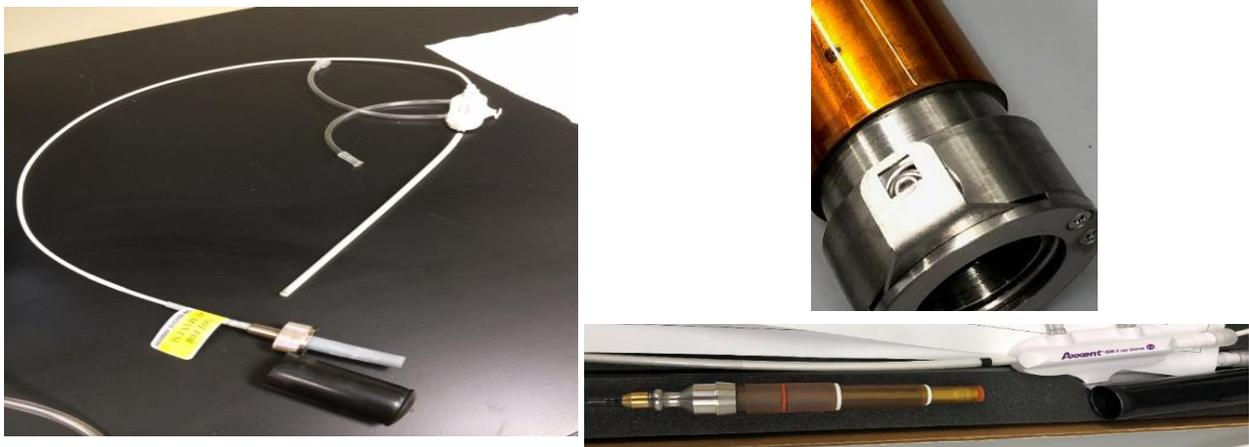
Figure 1b. The Xofter Axxent miniature x-ray S7500 water cooled source and threaded HV connector on left and the S7500/S7600 click HV connector with socket, on right.
