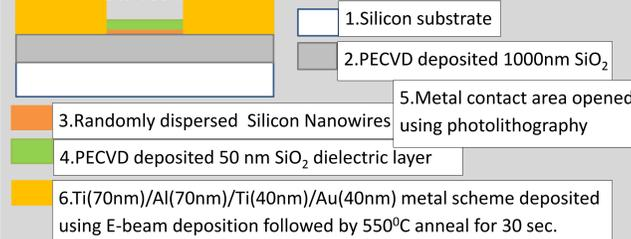
Figure 3. FET Fabrication process flow
