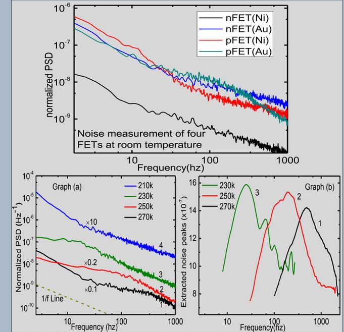
Graph (a) shows the temperature dependent noise measurement done on a single FET device. Evolution of Lorentzian behavior from low to high temperature is clearly obvious. Graph (b) show the peaks, extracted from the data of graph (a). It clearly depicts how the peak shifts in frequency with changing temperature.
