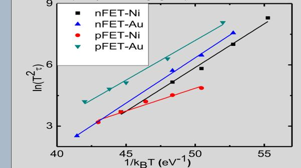
$\ln(T^2\tau)$  vs.  $1/k_B T$  plot for four FET devices (equations 1 and 2). Table shows all the computed values from this plot.
