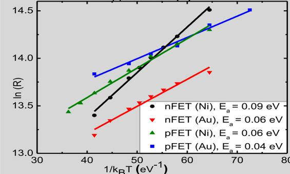
Arrhenius plot confirmed semiconducting behavior of the devices. Activation energy was computed using eq:  $\ln(R) = \ln(R_0) + E_a/2k_B T$  (where  $R_0$  is the intercept,  $E_a$  is the activation energy,  $k_B$  is the Boltzmann's constant, and T is absolute temperature). No information related to deep levels could be inferred from this data.
