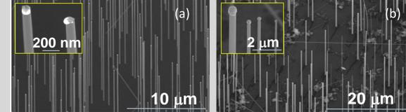
Au-catalyzed SiNWs were grown at 900 °C for 10 min. Average diameter of these NWs is about 130 nm. Ni-catalyzed SiNWs were grown at 1000 °C for 5 min. Diameters of these NWs varied between 100 nm and 600 nm
