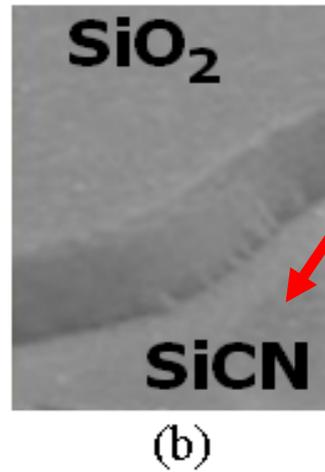
SEM image showing the SiO<sub>2</sub>/SiCN delamination (part of SiO<sub>2</sub> films are gone).
