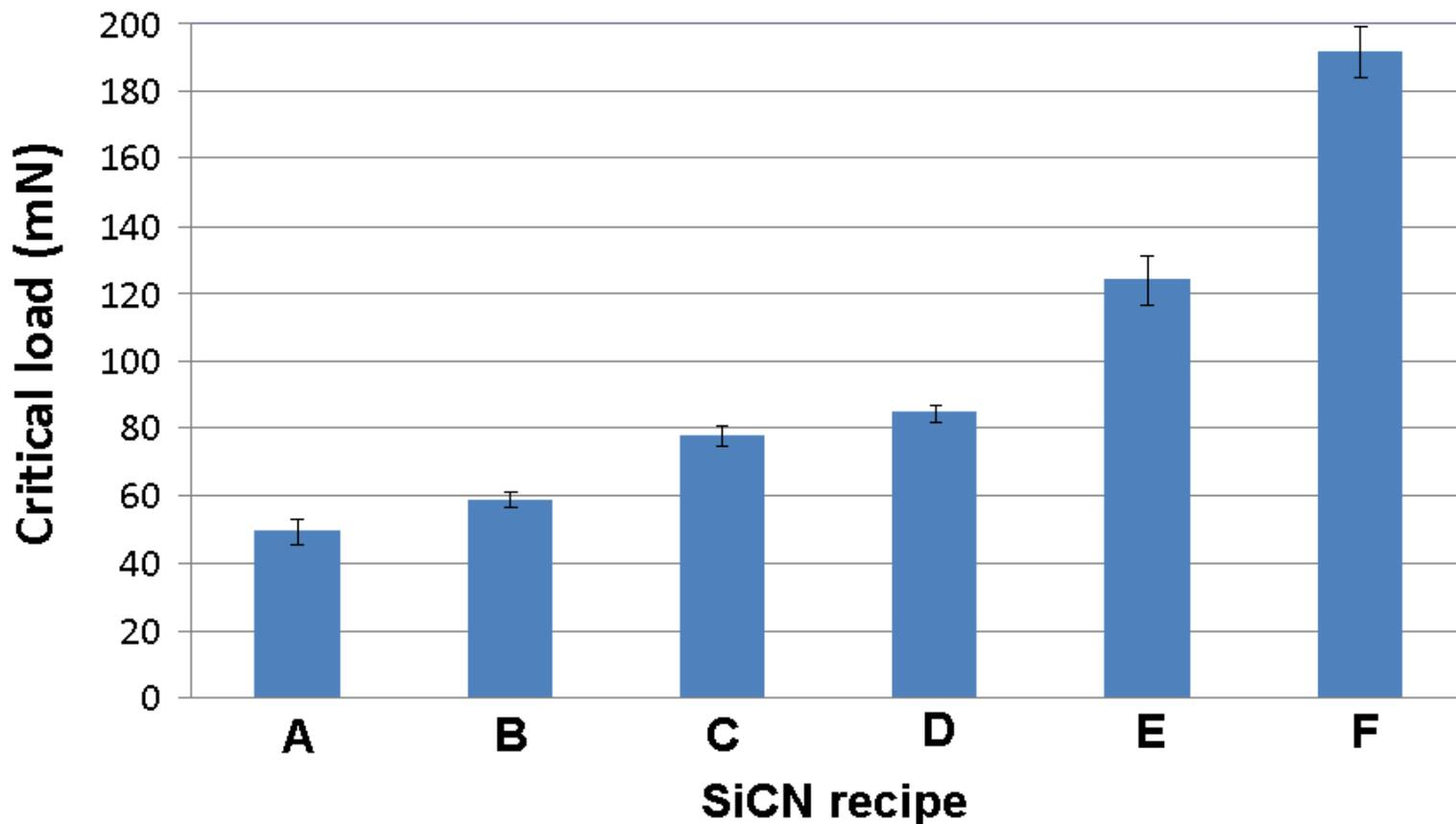
➤ By changing the SiCN deposition process, the SiCN/SiO<sub>2</sub> adhesion was significantly improved from sample A to F, as shown in both the optical images and critical loads.
