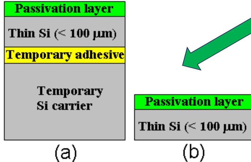
Wafer stack seen during the TSV integration process
