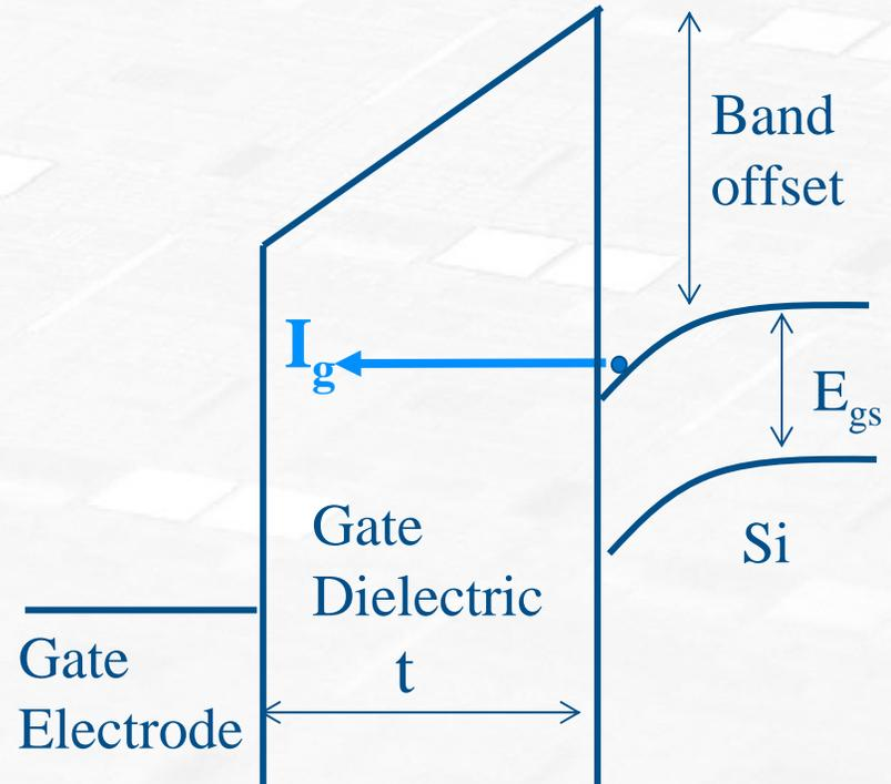
Requirement: Increase  $I_{sat} \propto \mu \cdot \epsilon / t$  without increasing  $I_g \propto \exp(-t\phi^n)$
