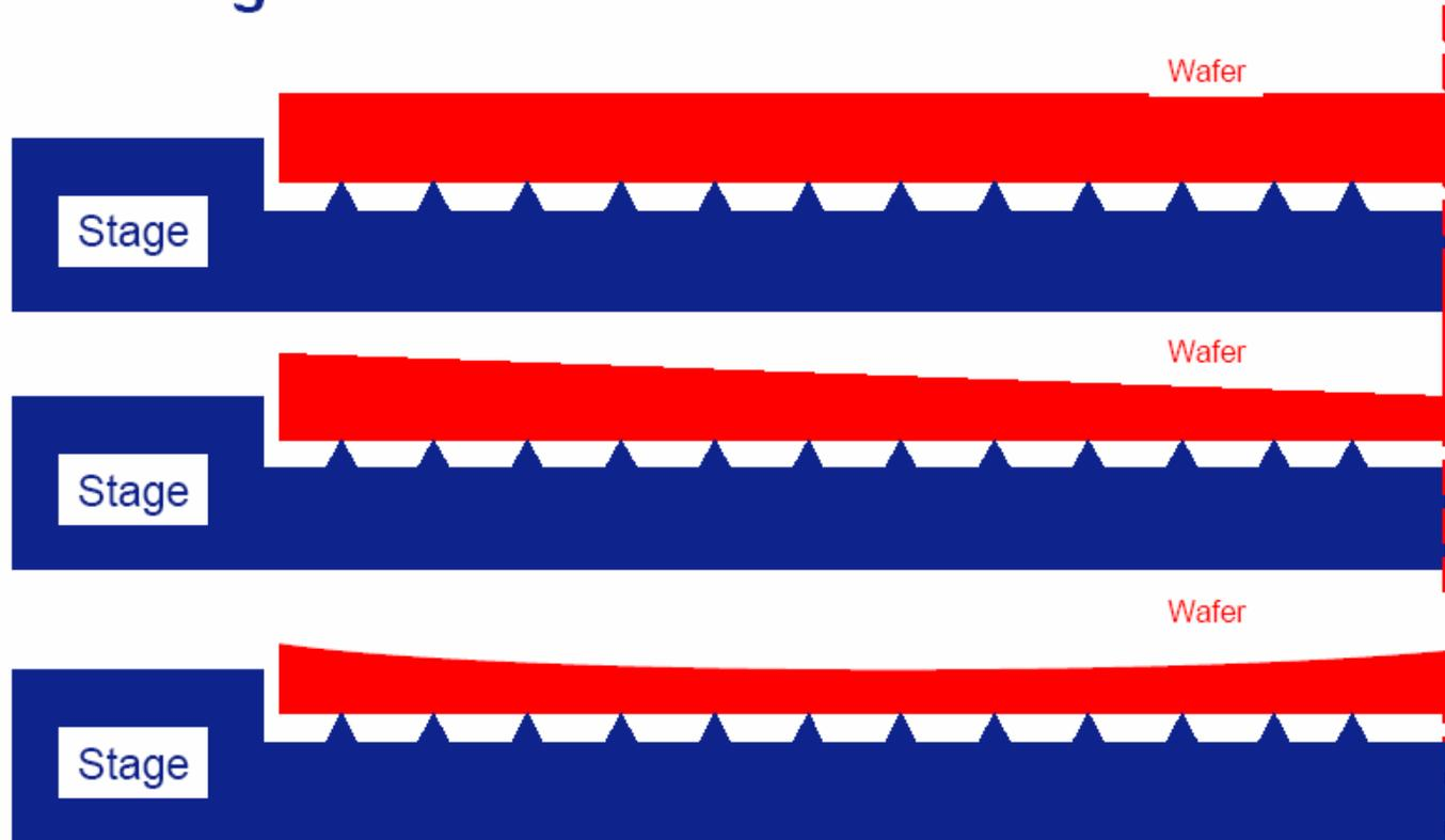
The wafer thickness at the edge must be very well controlled to maintain a homogeneous water film
