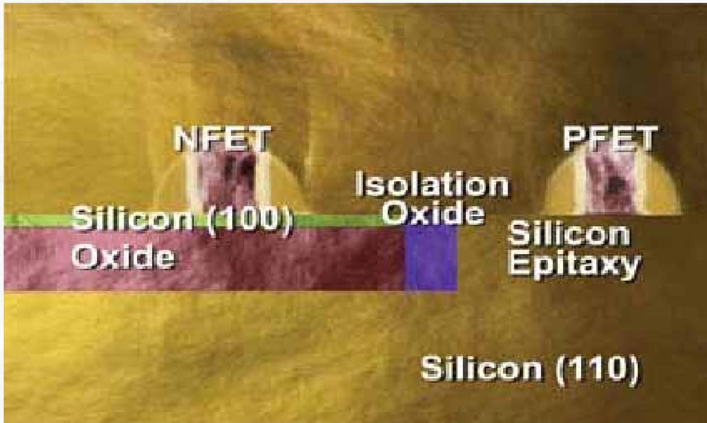
Hybrid Orientation Technology (HOT). PFET on (110) surface and nFET on (100) surface. Planar structure, fully compatible with standard CMOS processes. Reproduced with permission of Min Yang et al., (IBM) and the IEEE (© 2003 IEEE).
