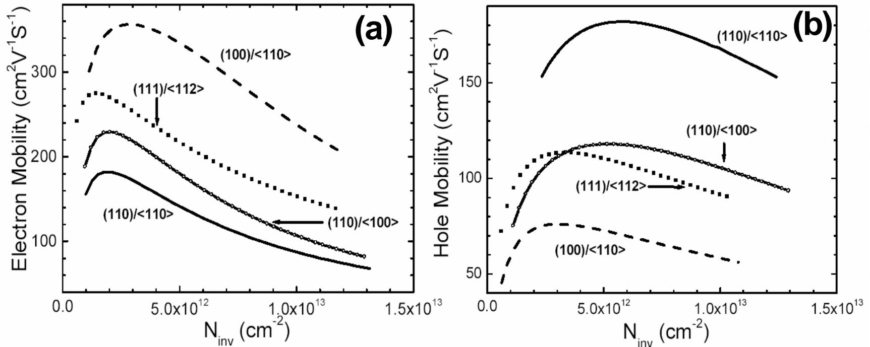
Orientation effect on the (a) effective electron mobility, (b) effective hole mobility as a function of inversion carrier density. Electron mobility is the highest on the (100) surface while the hole mobility on the (110) surface is more than 2.5 times higher than that on the (100) surface. Reproduced with the permission of M. leong et al., (IBM) and The Electrochemical Society, Inc.
