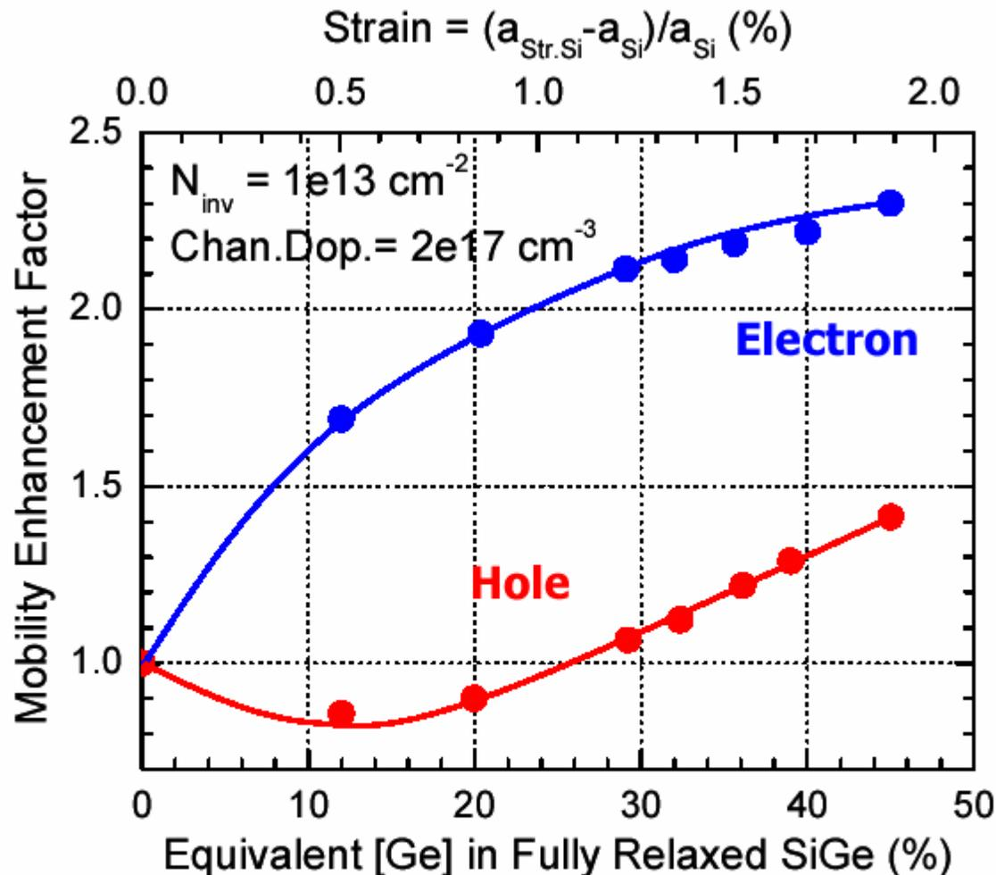
**Fig. 4.** Mobility enhancement vs. strain and [Ge] in strained Si/relaxed SiGe MOSFETs at  $1e13 \text{ cm}^{-2}$  carrier concentration. Hole mobility enhancement requires large amount of strain.
