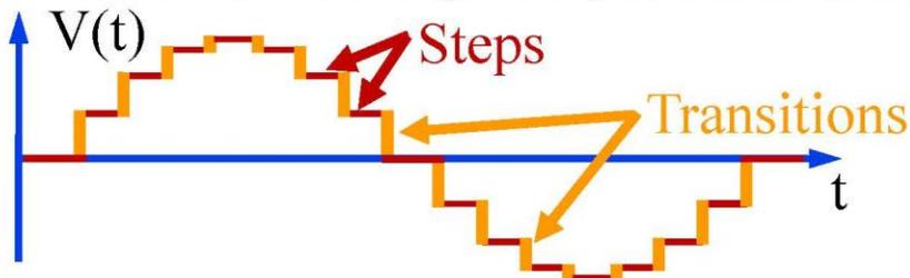
JAWS direct digital synthesis with current pulse sequences
