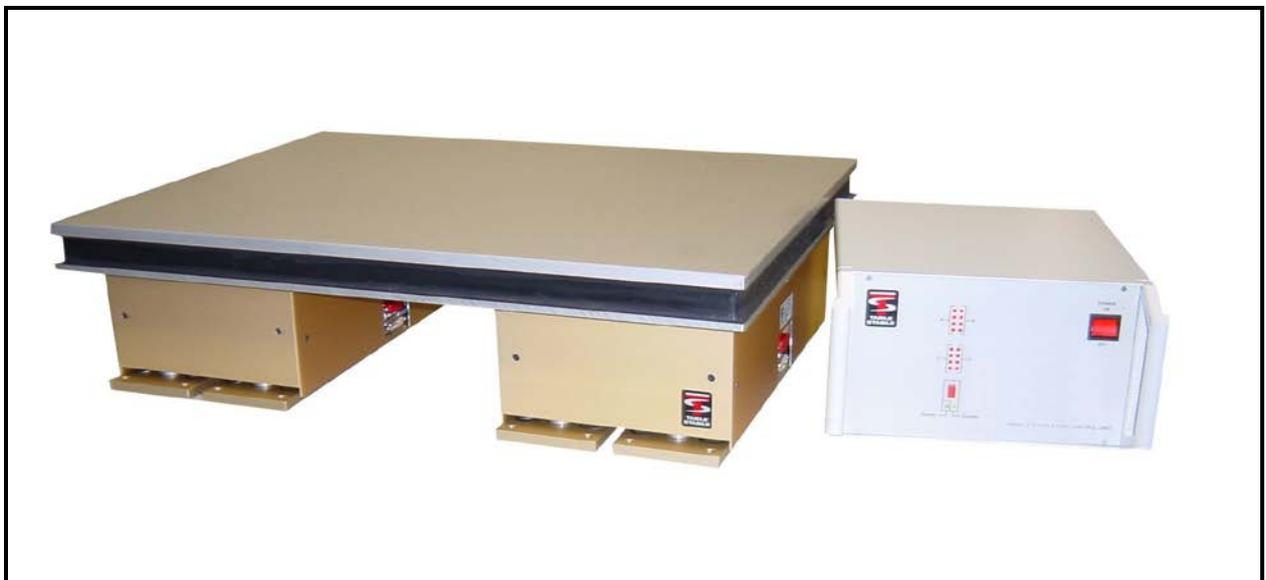
AVI-400/LP is an adaptable system consisting of two modules and is ideal for supporting delicate Fabry-Perot interferometers and tunnel-microscopes, allowing the ultimate performance to be achieved from these and other high resolution instruments. The tables have also proved to be extremely successful for supporting sensitive experiments, such as the troughs for liquids used in measurements on Langmuir-Blodgett films.
