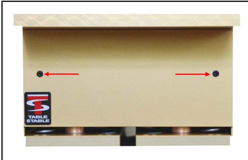
To expose the adjustment nuts, remove the end covers by undoing the screws shown in Fig. 3 (2mm hex key).
