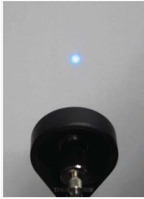
Single mode - looks Gaussian (sometimes hexagonal pattern of spots is visible around the central mode), smaller in size, smooth and not speckled. Not sensitive to fiber being jiggled.
