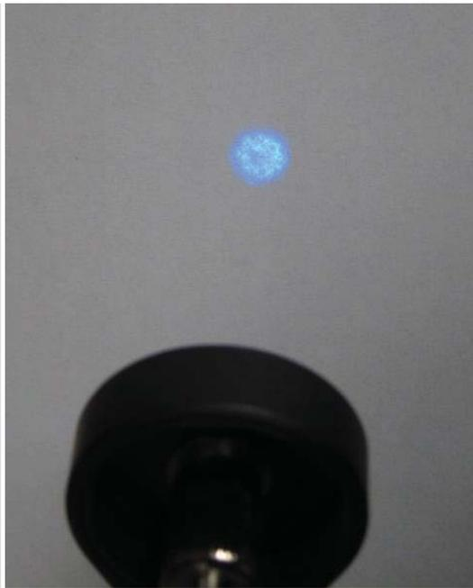
Speckle mode - note larger diameter/beam spread and speckled quality. Very sensitive to fiber jiggling.
