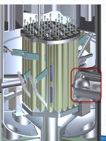
Existing hydrogen cold source is being replaced with more efficient deuterium cold source
