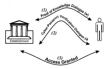
Registrant proves possession of working code w without exposing it; establishing a secure communication line based on w, in which the un-stored cyber-passport (u) is passed to the establishment, which verifies it based on its verification code,(v), not the cyber-passport itself.
