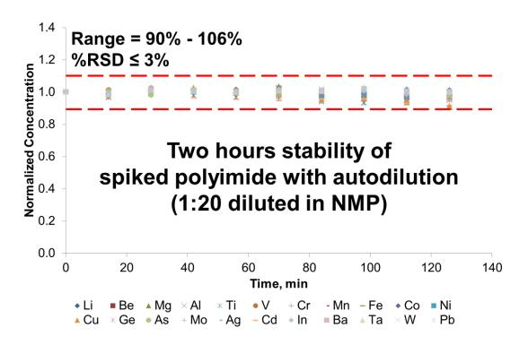
Two hours stability is plotted for a 5 fold inline auto dilution of 4 fold manually diluted and spiked polyimide.
