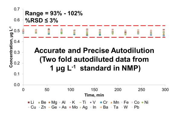
Twelve replicate analysis of a 2 fold auto dilution of 1 µg L<sup>-1</sup> in N-methyl-2-pyrrolidone ran over an 5 hours period demonstrate accuracy and precision of both standardization and replicate analysis. The signal stability was less than 3% and the accuracy was less than 10% for all elements during the period in spite of the complex organic matrix.
