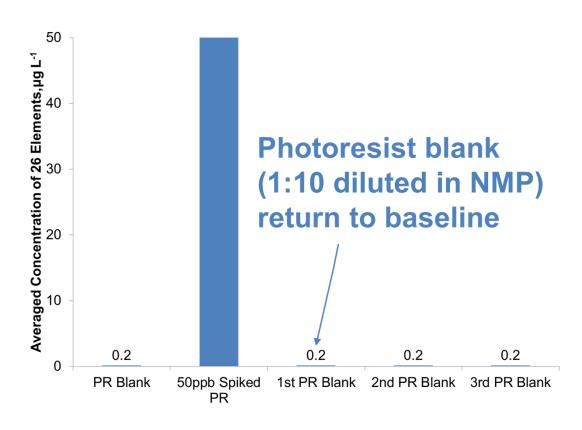
The blank concentration level in photoresist goes back to the previous baseline level at the fist blank after 50 µg L<sup>-1</sup> spiked photoresist analysis with prepFAST system. (Eements; Li, Be, B, Na, Mg, Al, K, Ti, V, Cr, Mn, Fe, Co, Ni, Cu, Zn, Ge, As, Mo, Ag, Cd, In, Ba, Ta, W and Pb)
