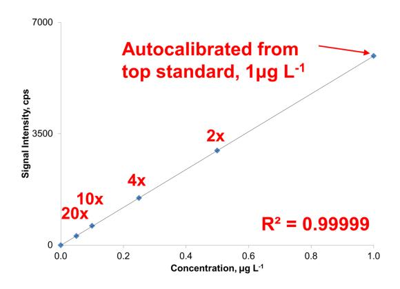
User predefined dilution factors for a single multi-element standard of 1  $\mu$ g L<sup>-1</sup> in N-methyl-2-pyrrolidon are used to build calibration curves. Accuracy of dilution is illustrated by excellent linearity of the calibration curve (R<sup>2</sup> = 0.99999).
