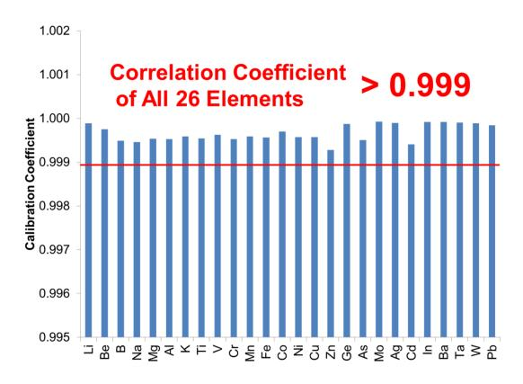
Twenty six potential contaminant elements in N-methyl-2-pyrrolidon were auto-calibrated from a single 1 µg L<sup>-1</sup> multielement standard solution. Autocalibration replicated 10 times and the averaged correlation coefficient of all elements exhibit better than 0.999 R<sup>2</sup> valvue.
