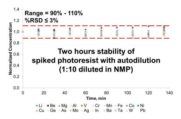
Two hours stability is plotted for a 10 fold inline auto dilution of spiked photoresist. These data indicates that undiluted photoresist can simple be placed in a tube and diluted inline to appropriate TDS for ICPMS analysis.
