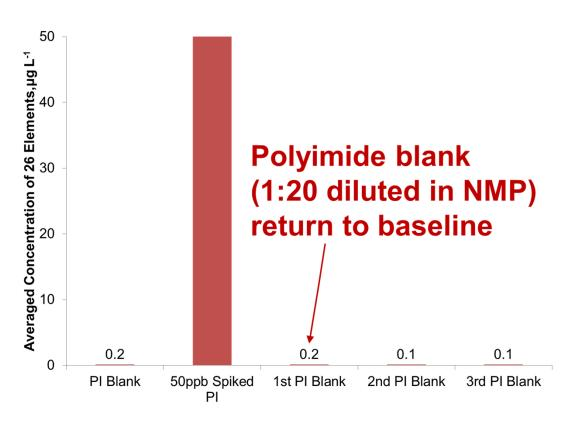
The blank concentration level in polyimide goes back to the previous baseline level at the fist blank after 50 µg L<sup>-1</sup> spiked polyimide analysis with prepFAST system. (Eements; Li, Be, B, Na, Mg, Al, K, Ti, V, Cr, Mn, Fe, Co, Ni, Cu, Zn, Ge, As, Mo, Ag, Cd, In, Ba, Ta, W and Pb)
