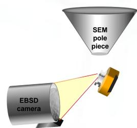
Conventional EBSD specimen-detector configuration, showing a sample tilted to 70° from horizontal.
