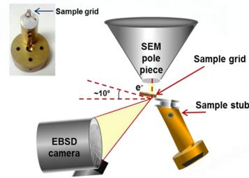
t-EBSD specimen-detector configuration. A simple custom specimen holder is used to hold a sample at 10° to 20° from horizontal.
