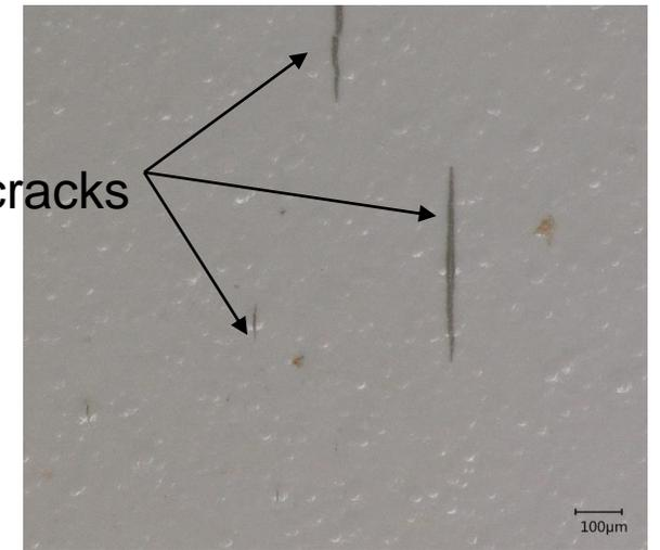
cracks form and extend along and beyond tabbing ribbons with additional thermal cycling
