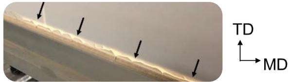
*new cracks and delamination*
