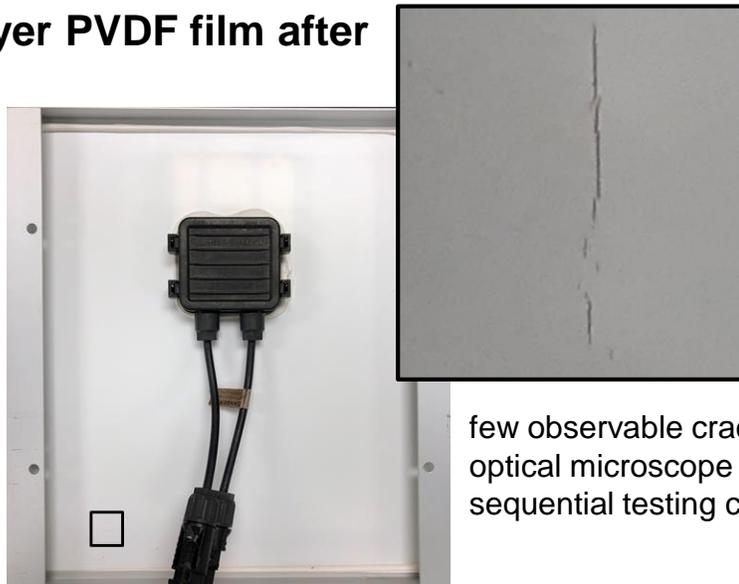
few observable cracks by optical microscope after single sequential testing cycle
