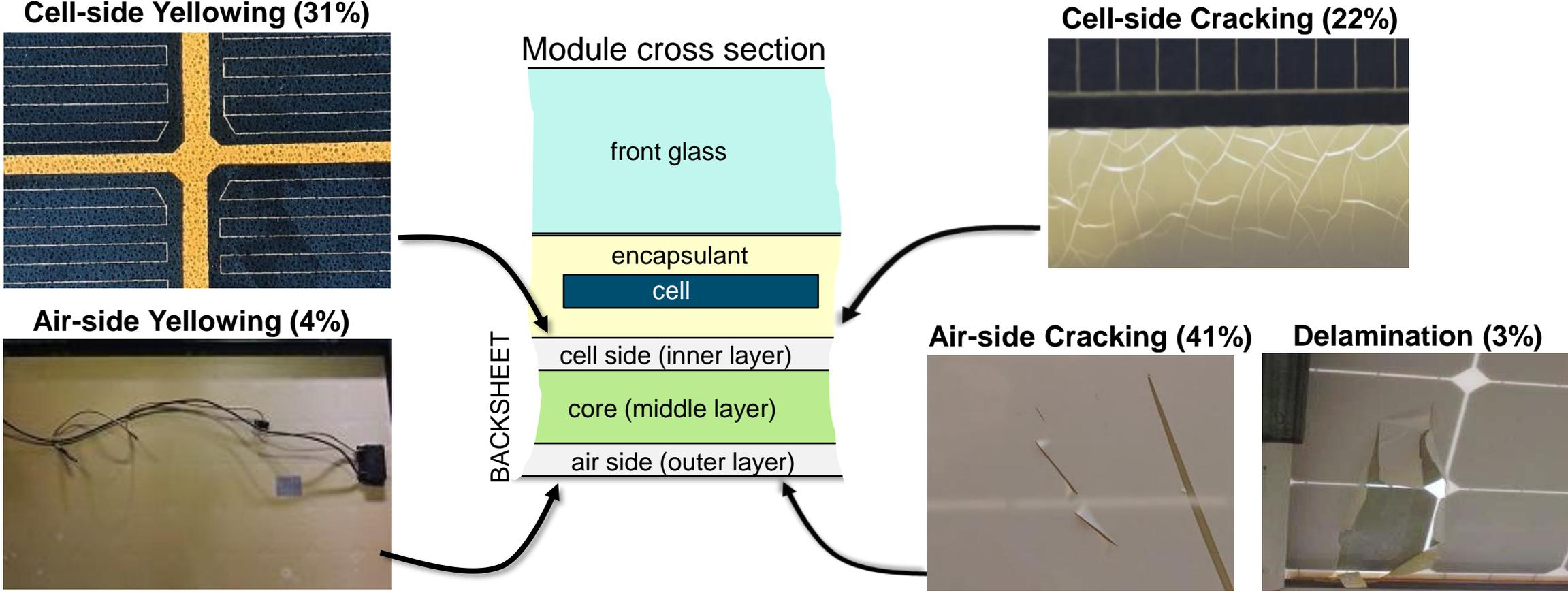
Cracking and delamination can compromise electrical insulation of the module
