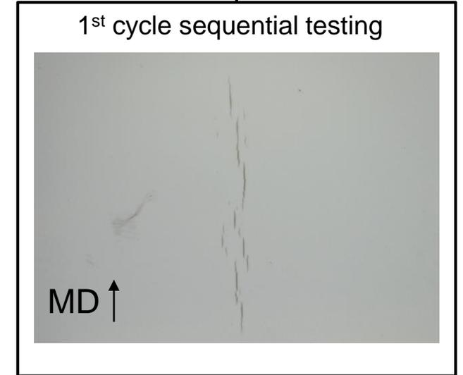
cracking along tabbing ribbon of single layer PVDF
