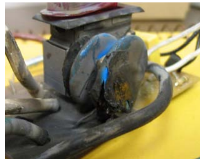
Figure 2 Crispy Factor CF2, indicating a flaky surface and some loss of physical structure
