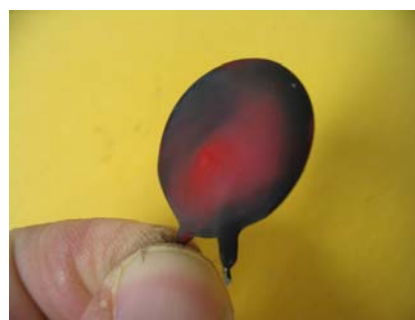
Figure 4 Crispy Factor CF0, indicating an intact MOV covered with soot from other MOVs
