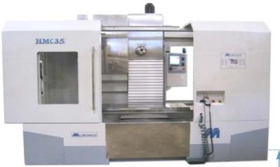
**Machine:** Milltronics HMC35, instrumented with sensors and data acquisition system
