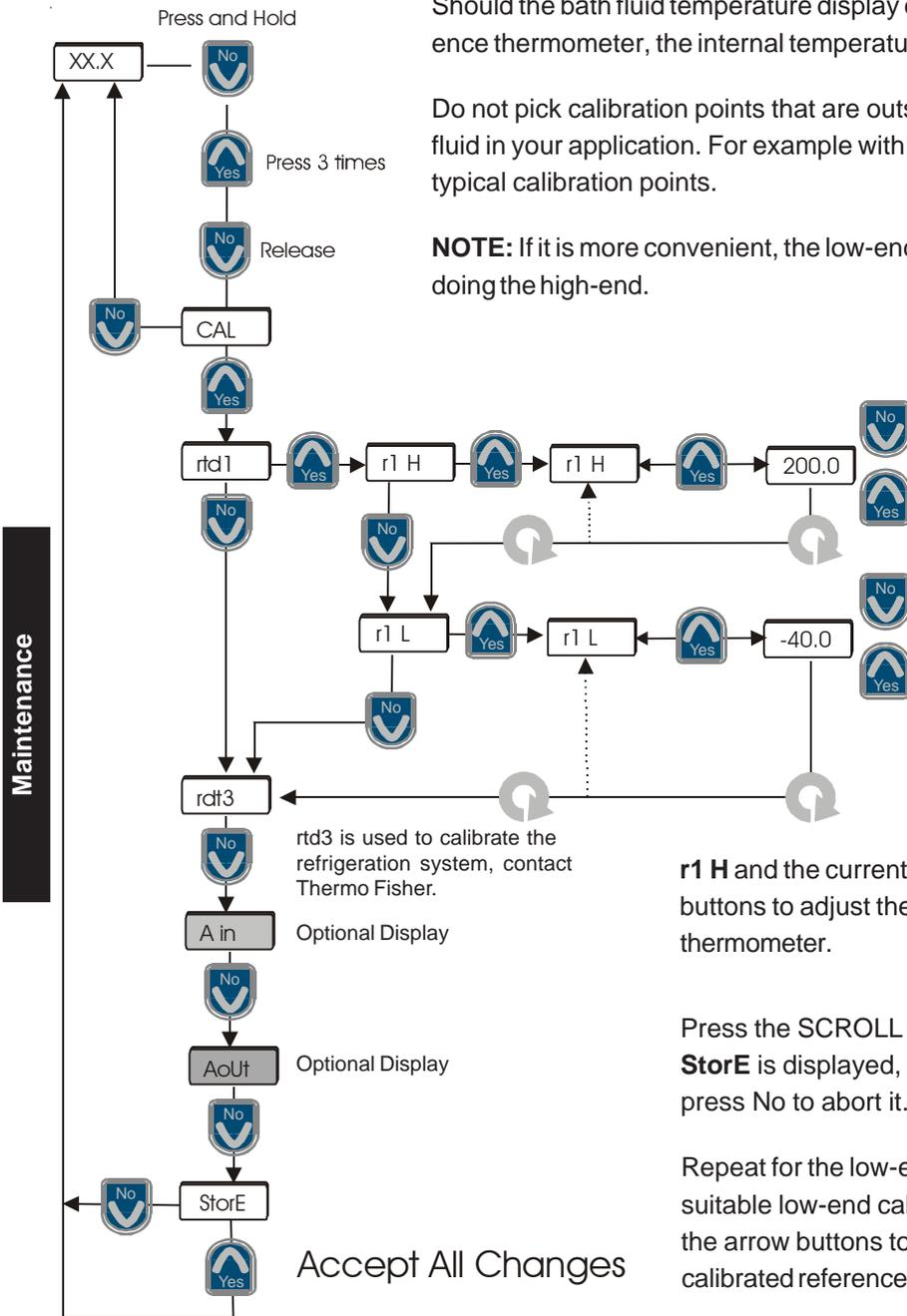
Should the bath fluid temperature display disagree with your calibrated reference thermometer, the internal temperature sensor (rtd1) may need calibration.
