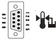
The unit is equipped with a male 9-pin D-connector located on the rear of the control box. The connector is used with an optional external sensor.
