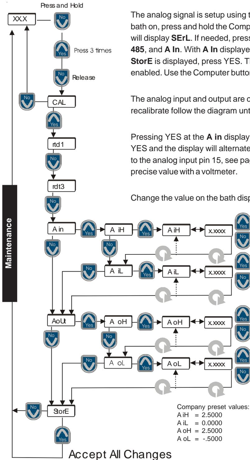
The analog signal is setup using the unit's Computer Setup Loop. With the bath on, press and hold the Computer button for five seconds. The controller will display **SErL**. If needed, press the arrow buttons to toggle between **232**, **485**, and **A In**. With **A In** displayed, press the Computer button again until **StorE** is displayed, press YES. The Computer button will flash when **A in** is enabled. Use the Computer button to enable/disable the analog signal.
