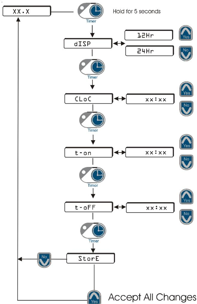
**NOTE:** Enabling serial communications disables the TIMER mode. If an error condition exists: serial communications enabled; time-on not defined; time-off not defined; or clock not set, the unit will beep and will not enable the function. The display will then indicate the reservoir fluid temperature.
