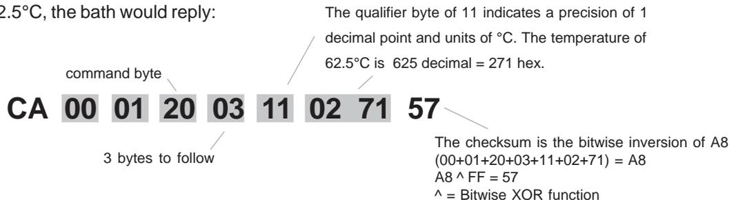
The master sets parameters in the bath by sending one of the Set Functions as shown in Table 1. The master does not send a qualifier byte in the data field. The master should be pre-programmed to send the correct precision and units (it could also read the parameter of interest first to decode the correct precision and units needed).
