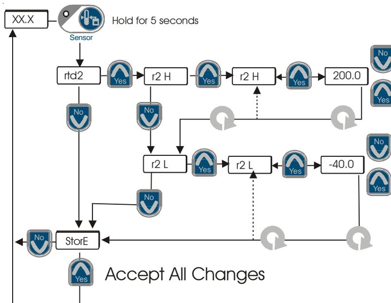
**NOTE:** If it is more convenient, the low-end calibration can be performed before doing the high-end.
