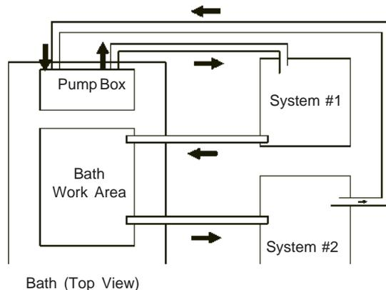
The pump can be used to circulate through two closed-loop systems. Connect the shortest practical length of flexible tubing from the pump outlet to the inlet of external system #1. Connect the outlet of system #1 directly into the bath work area. Connect tubing from the bath work area to the inlet of system #2. Connect the outlet of system #2 to the pump inlet.
